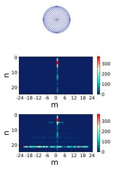
FIG. 2. (Top) points on a Lebedev sphere, and (Middle) reconstructed BSC for an incident focused vortex beam without noise and (Bottom) with 5% noise. (color online)
