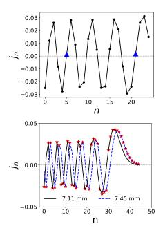
FIG. 3. (Top) Amplitude of the spherical Bessel  $j_n(kr)$  function for a radius  $r = 7mm(5.6\lambda)$  (the blue triangles show the values close to zero) and (Bottom) for two different radii  $r_1 = 7.11mm(5.7\lambda)$ and  $r_2 = 7.45(6\lambda)$  (the red points show the maximum values between  $|j_n(kr_1)|$  and  $|j_n(kr_2)|$  for each order n). The frequency is  $f_0 = 1.2MHz$ . (color online)
