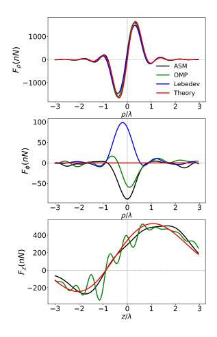
FIG. 11. Experimental radial  $F_{\rho}$ , azimuthal  $F_{\phi}$  and axial  $F_z$  forces exerted on an polystyrene sphere of radius  $r = 0.1\lambda$  in a focused Gaussian beam with charge m' = 0. (color online)
