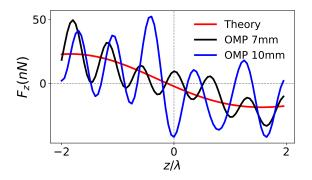
FIG. 9. Axial force exerted on a polystyrene sphere of radius  $r = 0.1\lambda$  with BSC computed by OMP method on two spherical surfaces (black and blue) and the theoretical force (red). (color online)
