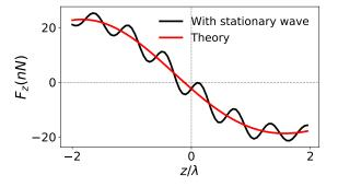
FIG. 8. Axial force exerted on a polystyrene sphere of radius  $r = 0.1\lambda$  with theoretical BSC  $A_n^m$  (black) and theoretical BSC with a counter propagating wave with 0.5% amplitude (red). (color online)
