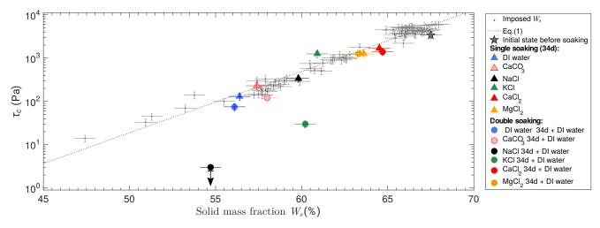
Fig. 7 Sediments yield stress  $\tau_c$  as a function of the solid mass fraction  $W_s$  after single soaking (triangles), double soaking (circles), or for prescribed solid mass fraction (black dots). pCO<sub>2</sub>=0.035%, solution volume is 20 cm<sup>3</sup> (the arrow below the black circle means that only a higher bound of the yield stress could be determined).
