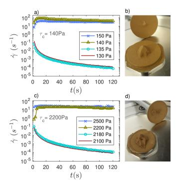
Fig. 3 Determination of the sediment yield stress. Shear rate as a function of time for different imposed stresses (see legend) for  $W_s = 57.7\%$  (a) and  $W_s = 66.0\%$  (c). Deposit shape after rheological measurement and upper plate removal for  $W_s = 57.7\%$  (b) and  $W_s = 66.0\%$  (d).
