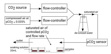
Fig. 5 Soaking experimental set-up.
