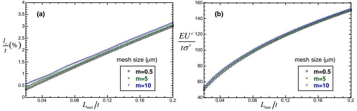
Figure 7: a) Initiation length and b) Applied displacement determined with the FFE approach versus the characteristic length for different values of the minimum mesh size  $m_{\text{FFE}}$  at the notch tip with  $M_{\text{FFE}} = 200\mu\text{m}$ . The three-point bending geometry with a sharp V-notch is considered with  $2L = 40\text{mm}$ ,  $w = 2\text{mm}$ ,  $h = 0.3\text{mm}$ ,  $\beta = 40\text{deg}$ . and  $E=400\text{ GPa}$ ,  $\nu = 0.2$ .
