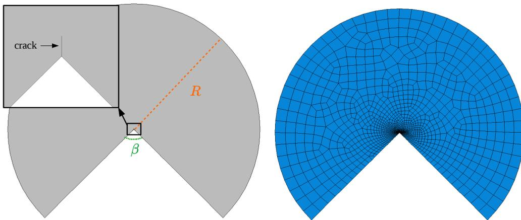
Figure 3: Inner domain of radius  $R$  in the case of a V-notch with angle  $\beta$  containing a unity length crack and an example of mesh employed for the computation of the energy difference (MA approach).
