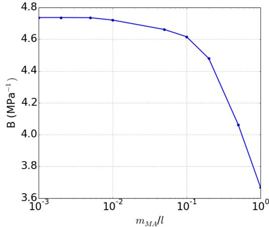
Figure 5: Coefficient  $B$  (MA approach) versus the minimum mesh size to crack length ratio  $\frac{m_{MA}}{l}$  for a sharp V-Notch with  $\beta = 90\text{deg.}$ ,  $E = 3300\text{MPa}$ ,  $\nu = 0.36$ . The inner domain radius to crack length ratio is  $\frac{R}{l} = 200$ .
