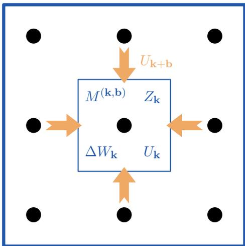
FIG. 2: Illustration of the parallelisation scheme for a  $3 \times 3$  mesh of  $k$ -points (black dots) and one MPI process per  $k$ -point. The calculation of the  $M^{(k,b)}$ ,  $Z_k$ ,  $\Delta W_k$  and  $U_k$  matrices are distributed over processes by  $k$ -point. The  $U_{k+b}$  matrices for the neighbouring  $k$ -points are sent from process to process (orange arrows) for the calculation of the  $M^{(k,b)}$  and  $Z_k$  matrices.
