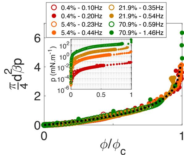
FIGURE 3. Normalized granular pressure obtained from the mixture model for a range of frequencies and density contrasts. Black dotted line corresponds to the analytical expression for the pressure as given by Eq. (6). The inset shows the non-normalized pressure in semi-log scale.
