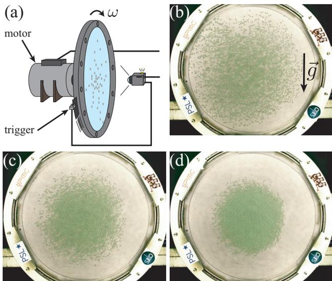
FIGURE 1. (a) Schematics of the experimental setup. (b)-(d) Snapshot of the system for a relative density contrast of  $\Delta\rho/\rho = 5.4\%$  at rotation frequencies 0.2Hz (b), 0.4Hz (c) and 0.6Hz (d).
