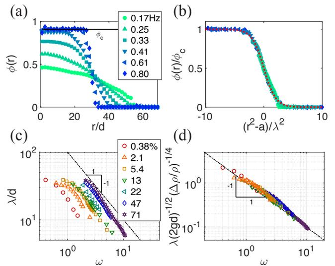
FIGURE 2. (a) Radial packing fraction for selected rotation frequencies  $0.17\text{Hz} < f < 0.8\text{Hz}$  at  $\Delta\rho/\rho = 5.4\%$ . The horizontal line locates the maximum fully crystalline packing fraction  $\phi_c$ . (b). Corresponding rescaled packing fraction profiles using the fitting function given by Eq. (1). (c) The fitting parameter  $\lambda$  as a function of  $\omega = 2\pi f$  and for different density contrasts. (d) Plot of  $\lambda$  rescaled using Eq. (3).
