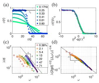
FIGURE 2. (a) Radial packing fraction for selected rotation frequencies 0.17Hz < f < 0.8Hz at  $\Delta \rho / \rho = 5.4\%$ . The horizontal line locates the maximum fully crystalline packing fraction  $\phi_c$ . (b). Corresponding rescaled packing fraction profiles using the fitting function given by Eq. (1). (c) The fitting parameter  $\lambda$  as a function of  $\omega = 2\pi f$  and for different density contrasts. (d) Plot of  $\lambda$  rescaled using Eq. (3).
