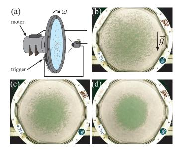
FIGURE 1. (a) Schematics of the experimental setup. (b)-(d) Snapshot of the system for a relative density contrast of  $\Delta \rho / \rho = 5.4\%$  at rotation frequencies 0.2Hz (b), 0.4Hz (c) and 0.6Hz (d).
