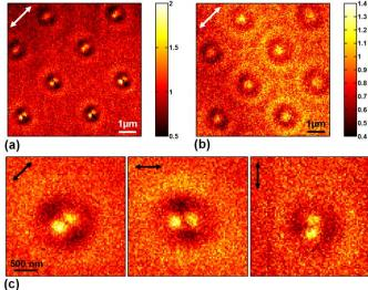
Figure 2: Fluorescence images measured at  $h_1$  = 0 nm (a) and  $h_2$  = 250 nm (b) above the 200 nm-diameter nanodisks (D200). Fluorescence images measured at  $h_1$  above one of these disks for different incident polarization directions (c).
