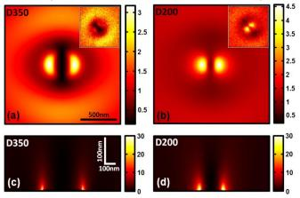
Figure 5: Near-field intensity calculated above D350 (a,c) and D200 (b,d). The simulation are performed in a plane parallel to the surface at  $h_S = 8$  nm (a,b) or in a plane perpendicular to the surface (c,d). The intensity was averaged on a 100 nm wide cube for (a) and (b). No average was made for (c) and (d). The insets represent the experimental images.
