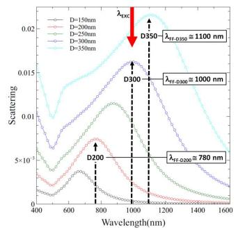
Figure 6: Scattering spectra of individual nanodisks calculated by FDTD. Our excitation wavelength  $\lambda_{EXC}$  is closer to the resonance wavelength of D350 ( $\lambda_{FF-D200}$ ) than the one of D200 ( $\lambda_{FF-D200}$ ). Nevertheless, the near-field fluorescence enhancement is larger for D200.
