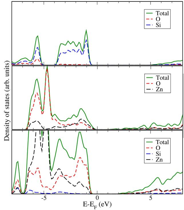
**Fig. 2** Local density of states (LDOS) of bulk  $\text{SiO}_2$  (top),  $\text{ZnO}$  (center), and  $\text{t-Zn}_2\text{SiO}_4$  (bottom) projected on zinc (black), silicon (blue) and oxygen (red) atoms.
