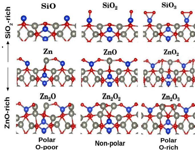
**Fig. 3** Atomic structures of the alternative terminations of the (001) surface. Left to right: oxygen lean to oxygen rich. Top to bottom: SiO<sub>2</sub> rich to ZnO rich. In each row, the central configuration is non-polar. Si, Zn, and O atoms are represented by large blue, large grey, and medium red balls, respectively.
