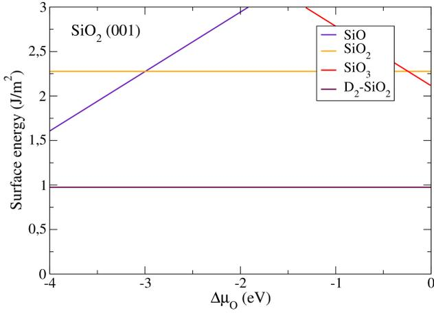
**Fig. 7** Calculated surface energies of the different terminations of the  $\text{SiO}_2$  (001) surface as a function of oxygen chemical potential  $\Delta\mu_{\text{O}}$ . The  $\text{D}_2\text{-SiO}_2$  termination is the reconstructed non-polar termination with two-membered siloxane rings. Adapted from Ref. 10.
