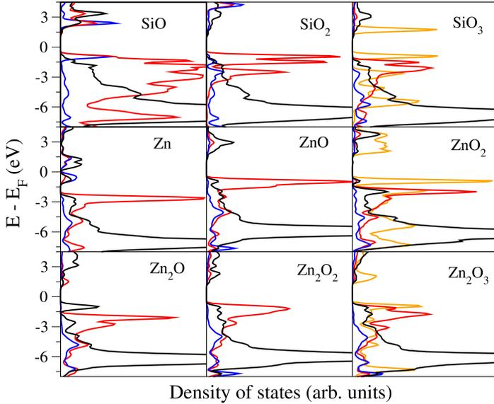
**Fig. 4** Local density of states (LDOS) at the (001) surface of  $t\text{-Zn}_2\text{SiO}_4$  projected on surface zinc (black), silicon (blue), and oxygen atoms (orange for peroxo groups, red for other surface oxygen atoms) at the nine terminations. Left to right: oxygen lean to oxygen rich. Top to bottom: SiO<sub>2</sub> rich to ZnO rich.
