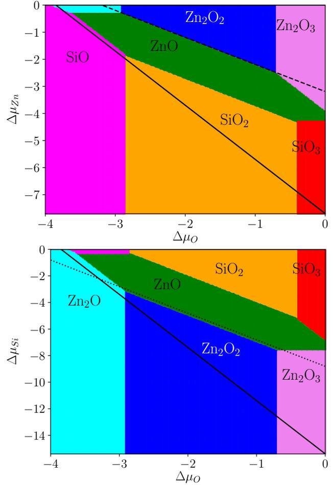
**Fig. 5** Surface stability of  $t\text{-Zn}_2\text{SiO}_4$ : most stable surface termination as a function of oxygen and zinc (top) and oxygen and silicon (bottom) chemical potentials. Solid diagonal lines represent  $\Delta\mu_{Si} = 0$  (top) and  $\Delta\mu_{Zn} = 0$  (bottom). The dashed (dotted) line in the top (bottom) panel corresponds to the equilibrium with bulk ZnO (SiO<sub>2</sub>).
