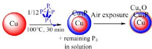
case of nickel, palladium, or iron, the crystallization of Cu<sub>3</sub>P was observed. Upon air exposure during the washing of the nanoparticles, a thin layer of copper oxide formed on the very external surface of the nanoparticles.
