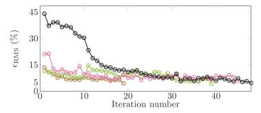
**Fig. 9.** Evolution of  $\epsilon_{\rm RMS}$  for three different cases (lines are guides to the eye): a box-like potential with length  $L=160~\mu{\rm m}$  (black), two box-like potentials separated by a barrier (brown), a box-like potential with a sinusoidally modulated bottom (green) and a V-shaped potential (pink). All initial and final densities and potentials are plotted in Figs. 7(a)-7(d).
