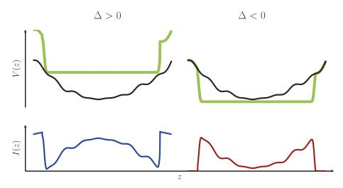
**Fig. 2.** Creating a box-like potential (green) by superposing blue- or red-detuned light fields ( $\Delta > 0$  and  $\Delta < 0$  respectively) with a rough harmonic potential (black). The intensity profiles needed to achieve the target potential is shown for each case.
