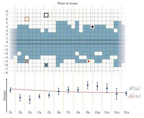
**Fig. 6.** Updating the DMD pattern based on the comparison between the averaged measured density,  $\bar{\rho}^i(z_k)$ , and the target density,  $\rho_T^i(z_k)$ . The process is explained in detail in the final part of Sec. 4. The example here shows a small longitudinal segment of iteration number i=14 of the optimization leading to the results shown in Fig. 7(c). The region on the DMD corresponds to an interval  $z_1=-39.89~\mu m$  to  $z_{13}=-26.23~\mu m$ .
