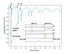
Figure 2: PD signal, propagation and attenuation. PD occurring at 70 m from the cable far end.
