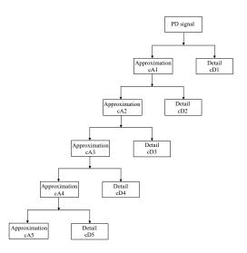
Figure 5: Block diagram of wavelet decomposition.
