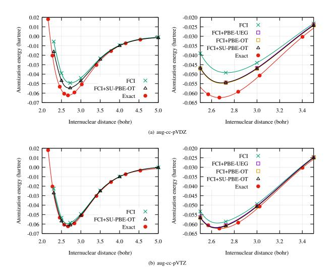
FIG. 4. Potential energy curves of the  $F_2$  molecule calculated with exFCI and basis-set corrected exFCI using the aug-cc-pVDZ (top) and aug-cc-pVTZ (bottom) basis sets. The estimated exact energies are based on a fit of experimental data and obtained from Ref. 89. The estimated exact energies are based on a fit of the non-relativistic valence-only CEEIS data extracted from Ref. 80.
