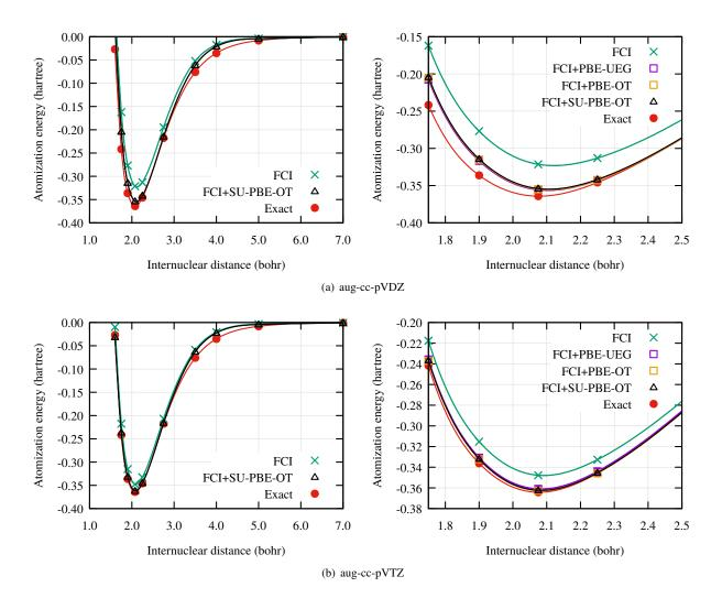
FIG. 2. Potential energy curves of the  $N_2$  molecule calculated with exFCI and basis-set corrected exFCI using the aug-cc-pVDZ (top) and aug-cc-pVTZ (bottom) basis sets. The estimated exact energies are based on a fit of experimental data and obtained from Ref. 89.
