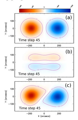
**Fig. 1.** Synthetic magnetograms of the axial (a) and the azimuthal (b) magnetic field components of a uniformly twisted torus model with  $N_{t,0} = 0.5$ . (c) Total superposed magnetic field map. The red- and blue-shaded areas represent the positive and the negative value of  $B_z$ . The magenta contour in each map corresponds to  $|B_z| = 50$  G (the maximum axial field is set to 1000 G). The associated movies are available online (fig1\_a.avi, fig1\_b.avi, and fig1\_c.avi).
