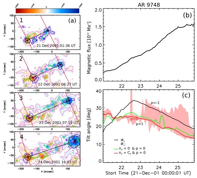
**Fig. 9.** (a) SOHO/MDI magnetograms of AR 9748. The magnetograms have the same contours and colour convention as Fig. 7a. (b) Evolution of the AR magnetic flux computed from the magnetograms (black line). (c) Evolution of  $\phi_a$  derived from the magnetic barycentres (black line) and  $\phi_c$  obtained from the core flux centres with the same coloured pattern and input parameters as the ones used in Fig. 7c. The associated movie is available online (fig9\_a.avi).
