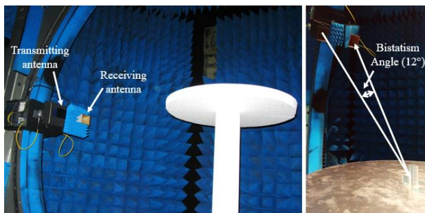
Figure 1: In the case of this picture the emitter and the receiver are moved on a semi-vertical arch during the scattering measurement in a quasi-monostatic configuration. The targets are placed on the metal disk supported by a polystyrene mast.
