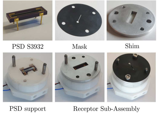
Figure 10. Receptor Sub-Assembly main elements. From left to right, from top to bottom: one-dimensional PSD S3932 by HAMAMATSU provides a photosensitive area of 1mm \times 12mm , a dark steel mask of 0.15mm thick, containing a slit, can be mounted on the ReSA support. The slit width equals 0.4mm and it is oriented perpendicular to the PSD photosensitive area, dividing it into two halves. Aluminum shims of 2.5mm height allow to position the slit at a distance d_B from the PSD surface.
