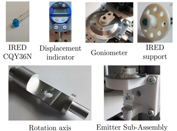
Figure 11. Emitter Sub-Assembly main elements. From left to right, from top to bottom: IRED CQY36N from Vishay provides a wide half-intensity emission angle \varphi = \pm 55^\circ , a displacement indicator ROCHPROFIL of 0.01mm resolution allows to measure translations on each axis, a goniometer allows to quantify the rotation on the vertical axis, the IRED support can be rotated around IRED's central axis by steps of 45^\circ , the rotation axis hosts the IRED support and its rotation axis is coincident with the IRED's chip. Finally the complete Emitter Sub-Assembly.
