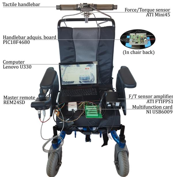
Fig. 1. Experimental setup.
