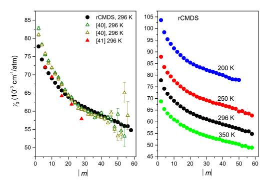
**Fig. 2**: Left panel:  $O_2$ -broadening coefficients of  $CO_2$  lines deduced from fits of rCMDS-calculated spectra at 296 K (black circles) with the sdNG profile and comparison with measured values of [40] (olive and dark yellow triangles for the  $30012 \leftarrow 00001$  and  $30013 \leftarrow 00001$  bands, respectively) and [41] (red triangles) (see text).
