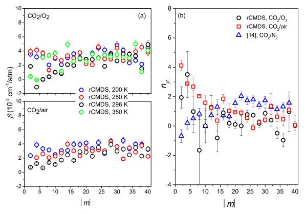
**Fig.** 7: Left panel: the rCMDS-predicted Dicke narrowing parameters for  $O_2$  and air-broadened  $CO_2$  for all the considered temperatures. Right panel: the deduced temperature exponents of the Dicke narrowing parameters for  $O_2$ - and air-broadened  $CO_2$  lines and comparison with measurement-deduced values of [14] for  $CO_2/N_2$ .
