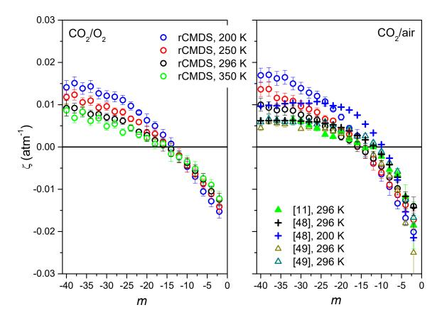
*Fig.8*: *Left panel: first-order line-mixing parameters predicted from rCMDS for O*<sub>2</sub>*-broadened CO*<sub>2</sub> *at 200, 250, 296 and 350 K.*
