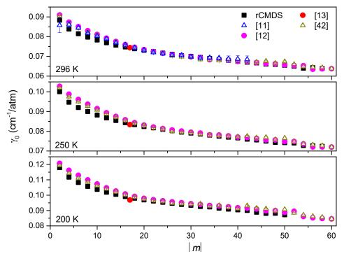
**Fig.3**: Air-broadening coefficients predicted by rCMDS using results obtained here for  $O_2$ -broadening and those for  $N_2$ -broadening obtained in [16] and in this study, at 296, 250 and 200 K. Results of [13], [11], and [12,42], obtained from fits of measured spectra with respectively, the sdNG, pcsdNG and sdV profiles, are also displayed for comparison.
