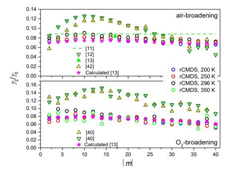
**Fig. 5**: Bottom panel: the ratio  $\gamma_2/\gamma_0$  predicted by fitting the rCMDS-calculated spectra of  $CO_2/O_2$  with the sdNG profile, obtained at 200 K, 250 K, 296K and 350K and comparison with the temperature-independent values of [40] (olive and dark yellow triangles) obtained from fits of measured spectra with the sdV profile. The temperature-independent values, calculated using Eq. (1) [13] and our temperature exponents (magenta stars) are also shown.
