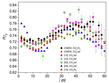
**Fig. 4**: The temperature exponents of  $O_2$ - (black circles) and air-broadening (olive circles) coefficients of  $CO_2$ , deduced from rCMDS and comparison with those for  $CO_2$  in air of [12] (purple diamonds), [13] (green triangles), [42] (olive triangles) and [44] (blue triangles) and for  $CO_2$  in  $N_2$  of [14] (red triangles).
