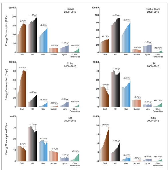
Figure 3. Average annual energy consumption (EJ) by fuel source from 2000 to 2018 globally and regionally, with average annual growth shown from 2013 through 2018 (BP 2019).
