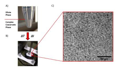
**Figure 4.** The complex coacervate phase, (**A**) liquid and transparent at low temperature and high ionic strength, turns into a white soft solid when exposed to either a temperature increase ( $\Delta T$ ) or (**B**) an ionic strength decrease ( $\Delta I$ ). (**C**) The solid material shows a porous structure due to the formation of water pockets.
