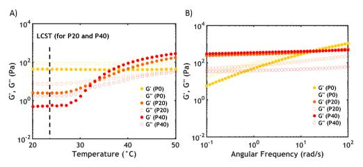
**Figure 9.** (**A**) Temperature sweeps and (**B**) frequency sweeps performed at 50 °C performed as a function of PNIPAM content for PxS0.75. Filled dots represent G', while hollow dots represent G''.
