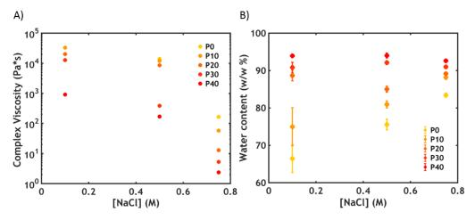
**Figure 2.** (A) Complex viscosity recorded at  $\omega = 0.1$  rad/s (P0S0.1 is missing since the measuring position in the rheometer could not be reached because of the high stiffness of the sample) and (B) water content at 20 °C as function of [NaCl] in PxSy. Error bars in (B) represent standard deviations.
