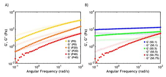
**Figure 3.** Frequency sweeps performed at 20 °C (**A**) for varying PNIPAM content for PxS0.75 and (**B**) as a function of [NaCl] for P40Sy. Filled dots represent G', while open dots represent G''.
