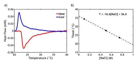
**Figure 6.** (**A**) Differential scanning calorimetry (DSC) thermogram for P40S0.75 and (**B**) *T<sub>heat</sub>* as a function of [NaCl] in P40Sy.
