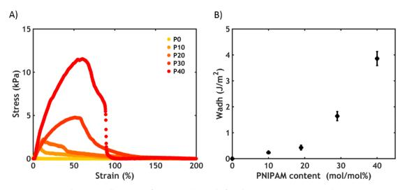
**Figure 11.** Underwater adhesion performance obtained after the temperature-activated setting process for the samples PxS0.75. (**A**) Stress-strain curves plotted in linear scale and (**B**) work of adhesion as a function of the PNIPAM content.
