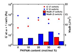
**Figure 15.** *G*' at  $\omega = 1$  rad/s and  $W_{adh}$  obtained after a temperature and a salt switch plotted as function of PNIPAM content.
