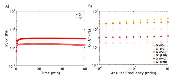
**Figure 13.** (**A**) Time sweeps performed on P40S0.75 and (**B**) frequency sweeps performed on samples PxS0.75 immediately after the salt-activation at 20 °C. Filled dots represent G', while hollow dots represent G''.
