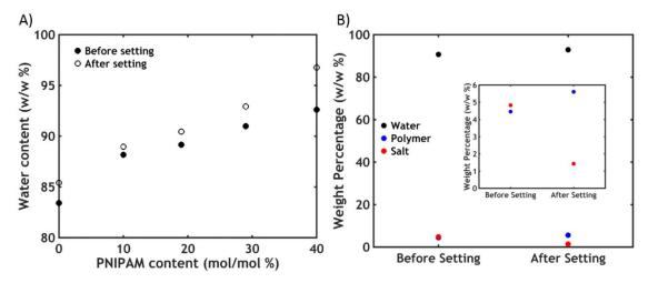
**Figure 12.** (**A**) Water content as a function of PNIPAM content for the samples PxS0.75 before and after the salt-activated setting process at  $T = 20 \degree C$ . (**B**) Water, polymer and salt content for the sample P30S0.75 before and after the setting process (a magnification of the lower part of the plot is reported in the inset).
