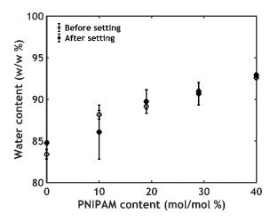
**Figure 8.** Water content as a function of PNIPAM content for the samples PxS0.75 before and after the temperature-activated setting process. Error bars represent standard deviations.
