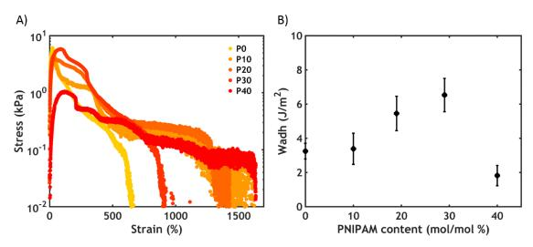
**Figure 14.** Underwater adhesion performance obtained after the salt-activated setting process for the samples PxS0.75. (**A**) Stress-strain curves plotted in log-lin scale and (**B**) work of adhesion as a function of the PNIPAM content.
