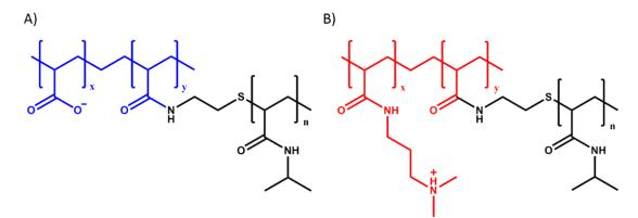
**Figure 1.** Molecular structure of (**A**) poly(acrylic acid) grafted with poly(*N*-isopropylacrylamide) (PAA-*g*-PNIPAM) and (**B**) poly(*N*,*N*-dimethylaminopropyl acrylamide) grafted with poly(*N*-isopropylacrylamide) (PDMAPAA-*g*-PNIPAM). The coloured parts represent the polyelectrolyte backbones while the black ones represent the PNIPAM units.
