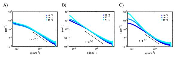
**Figure 7.** Small angle X-ray scattering (SAXS) plots at different temperatures for (**A**) P0S0.75, (**B**) P20S0.75 and (**C**) P40S0.75.
