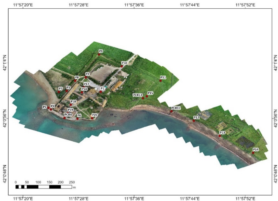
Figure 3. The orthophoto with the Ground Control Points (red dots) position used during the UAV surveys.
