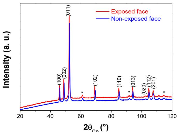
**Figure 2.** Experimental XRD patterns recorded on the directly exposed (red line) and non-exposed (blue line) to plasma implantation Ni pellet, within grazing conditions. Both were successfully indexed within the hexagonal  $\text{Ni}_2\text{H}$  structure (ICDD n° 98-020-1088). The small peaks marked by an asterisk correspond to the diffraction planes of the cubic Ni structure (ICDD n° 98-004-3397).
