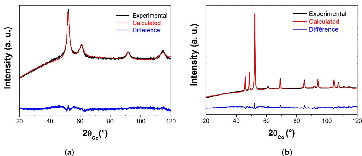
**Figure 1.** Experimental (black scatter) and calculated (red line) X-ray diffraction (XRD) patterns of polyol-made (a) and plasma treated (b) Ni powders. The residue, defined as the difference between the experimental and calculated diffractograms, is given (blue line) to illustrate the fit quality, with a Bragg reliability factor  $R_B$  ranging between 1.5 and 2.0.
