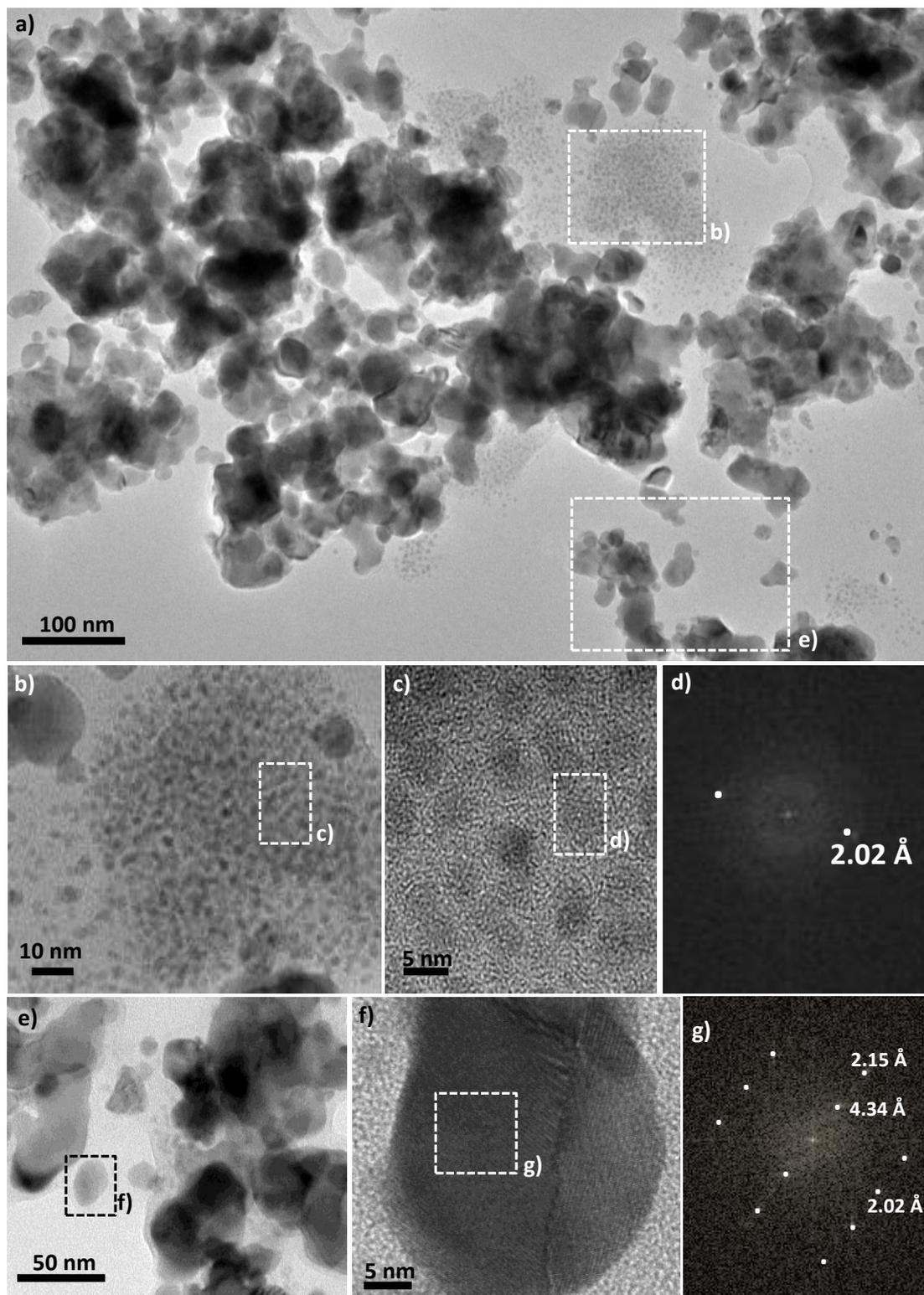
**Figure 4.** (a) TEM micrographs of the plasma treated Ni powder. Two populations of particles can be identified, the smallest and scarcest ones (b,c) and the largest ones (e,f). Fast Fourier transform (FFT) patterns calculated from high resolution TEM) images (c,f) recorded on representative particles of the two population are given and fully indexed within the fcc Ni structure (d) and the hc Ni<sub>2</sub>H one (g), respectively.
