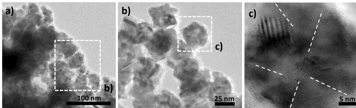
**Figure 3.** (a) Transmission electron microscopy (TEM) micrograph of the as-produced Ni powder. Only one population of particles can be identified: almost isotropic in shape polycrystals of 25–30 nm in size (b,c). More or less amorphous thin Ni hydroxide veils appear time to time around the Ni particles as a residual synthesis product (b). Note the white dashed lines are just guidelines.
