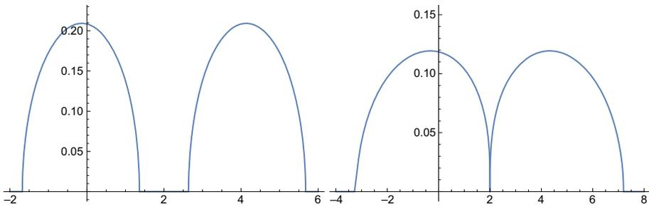
**Fig. 3** Density of states  $\rho(\lambda)$  for two coupled points,  $L = 2$ . We set  $t = 1$ . Left: weak disorder  $B''(0) = 0.3$ , the support splits in two disjoint intervals where the density of states is close to a semi-circle as for  $L = 1$ . Right: critical disorder  $B''(0) = 1$  at which the two interval touch
