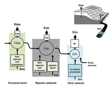
**Fig. 1** Principles of the model of N<sub>2</sub>O production and transfer through the land–river continuum. (Cbas, Crip and Criv stand for N<sub>2</sub>O concentration in the water phase of basin soil, riparian soil and river respectively; Sbas, Srip, Sriv are the suface area of watershed, riparian wetlands and river network.; Ebas, Erip,
