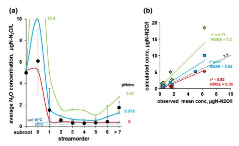
Fig. 4 Model-calculated average  $N_2O$  concentration in watershed and riparian water, as well as in surface water of different Strahler streams. Comparison with available measurements carried out in the Seine basin since 2012 (Garnier et al. 2009; Marescaux et al. 2018 and unpublished data). The level of  $N_2O$  saturation with respect to atmospheric concentration for two temperatures is also indicated (blue dotted lines:  $0.36 \mu gN-N_2O$
