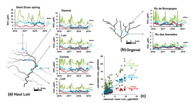
Fig. 2 Model-calculated time and space variations of  $N_2O$  concentration in river water of  $\bf a$  the Haut Loir basin and,  $\bf b$  the Orgeval basin, for three values of the pNden parameter (representing the fraction of total denitrification emitted as  $N_2O$  in riparian and stream processes).  $\bf c$  Scatter plot of
