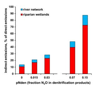
Fig. 5 Sensitivity analysis of the effect of pNden value on the model estimate of  $N_2O$  emissions by riparian and riverine processes in the Seine watershed
