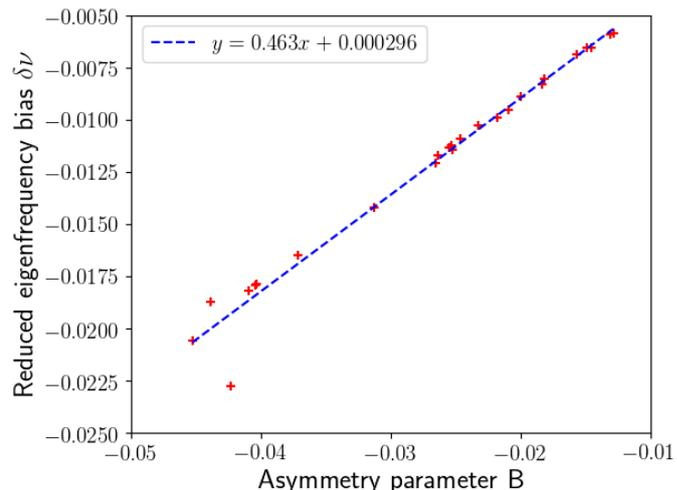
**Fig. 14.** Reduced frequency bias  $\delta\nu$ , defined by Eq. (34), as a function of the asymmetry parameter  $B$  for each radial  $p$ -mode between  $n = 6$  and  $n = 30$ . The blue dashed line shows the best linear fit.
