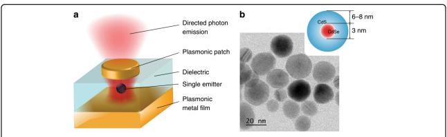
Fig. 1 A plasmonic patch antenna coupled to a single colloidal quantum dot. a Schematic of the structure under study consisting of a single colloidal core/shell QD coupled to a plasmonic patch antenna. b Schematic and transmission electron microscopy image of the investigated emitters
