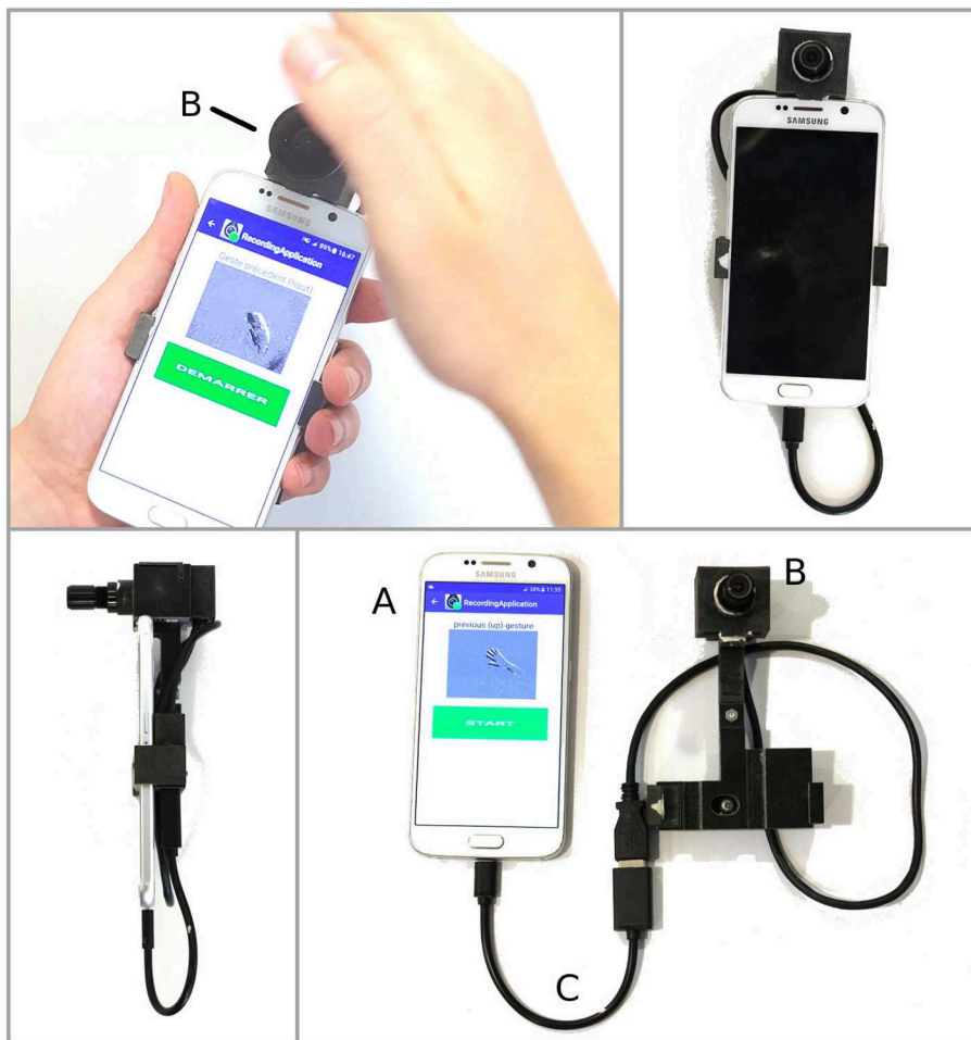
FIGURE 1 | A neuromorphic camera (an ATIS) (B) is plugged into a smart-phone (A) using an USB link (C), allowing mid-air gesture navigation on the smart-phone.
