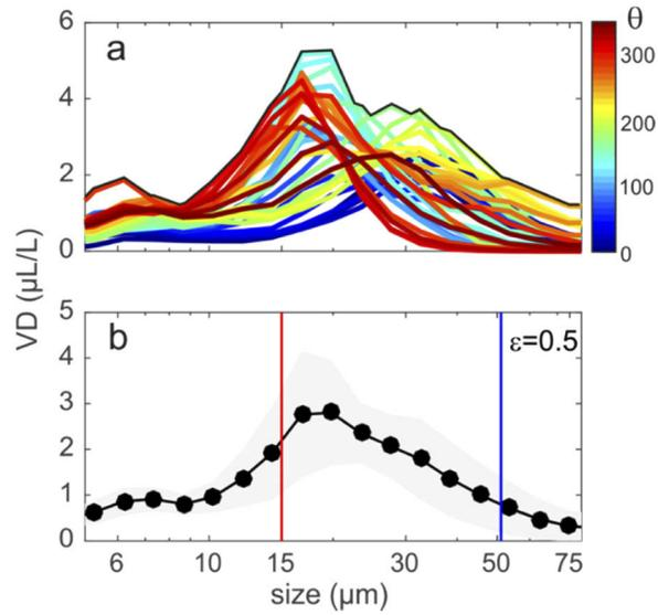
**Fig. 8.** a) Variation of the size spectrum with in-plane orientation  $\theta$  for  $\varepsilon=0.5$ . The black line represents the envelope. b) Mean spectrum. The red and blue lines represent  $a$  and  $b_{\perp}$  dimensions. The shaded area marks the mean  $\pm$  std.
