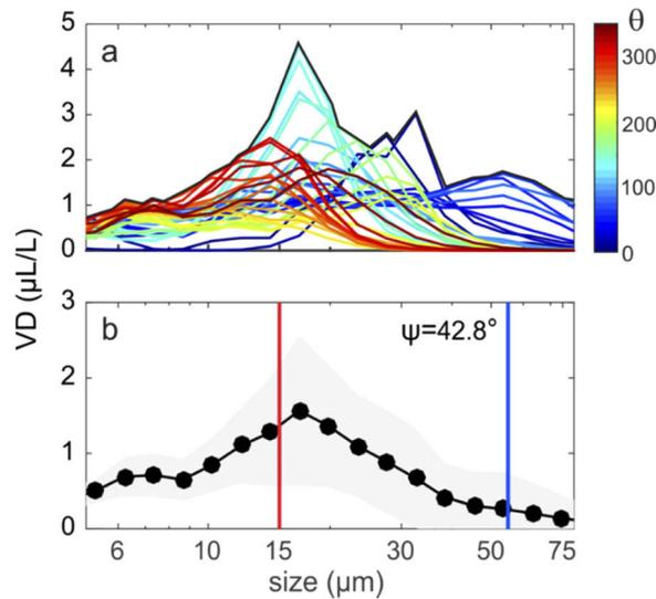
**Fig. 5.** a) Variation of the size spectrum with  $\theta$  alignment for  $\psi=42.8^{\circ}$ . The black line represents the envelope. b) Mean spectrum. The red and blue lines represent  $a$  and  $b_{\perp}$  dimensions. The shaded area marks the mean  $\pm$  std.
