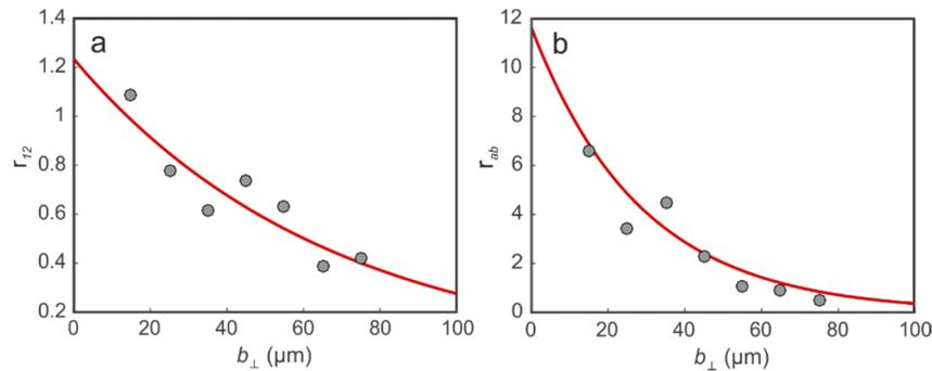
**Fig. 3.** a) The ratio of the diffraction signal  $r_{12}$  for the size of the minor axis ( $ch1=a$ ) and the size of the projected major axis ( $ch2=b_{\perp}$ ) of the micropillars with respect to  $b_{\perp}$  for the different orientations  $\psi$ . b) The ratio of the diffraction signal  $r_{ab}$  but for  $ch1=a$  and  $ch2=b$  as a function of  $b_{\perp}$ .
