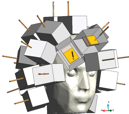
Figure 5. Computer-assisted design (CAD) model of the 3D microwave imaging system together with the anthropomorphic head phantom; two printed monopole antennas within the coupling medium bricks are highlighted in yellow.
