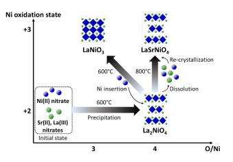
Scheme 2. Proposed mechanisms involved in the synthesis of nickel-based perovskites.
