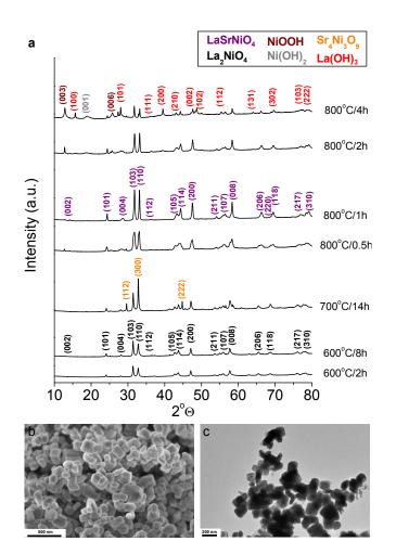
**Figure 3.** (a) XRD diagrams of the powders obtained at different temperatures and reaction times when targeting LaSrNiO<sub>4</sub> in NaNO<sub>2</sub>. (b) SEM and (c) TEM micrographs of LaSrNiO<sub>4</sub> obtained at 800 °C/1h.
