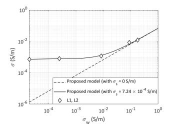
Figure 6: Electrical conductivity of two limestones  $(L_1 \text{ and } L_2)$  versus water electrical conductivity. The dataset is from Cherubini et al. (2019) and model parameters are given in Table 1.
