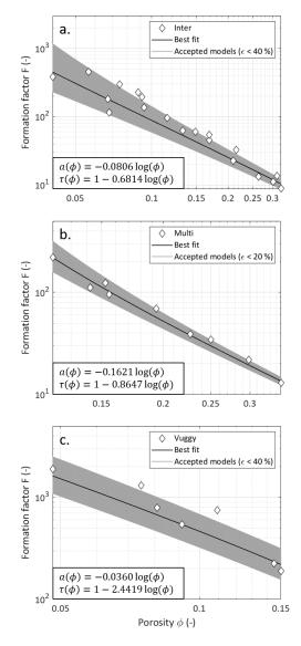
Figure 7: Formation factors of a set of carbonate rocks classified by pore types versus porosity. The dataset is from Garing et al. (2014). The model parameters are given in Table 1. The proposed model parameters are considered to be logarithmic functions of  $\phi$ . (a) "inter" stands for samples with intergranular pores (b) "multi" gathers samples with multiple porosity types: intergranular, moldic, and vuggy. (c) "vuggy" represents samples with vugular porosity.
