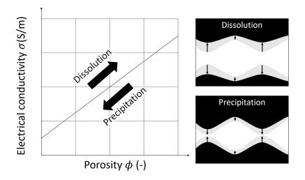
Graphical abstract: a new electrical conductivity model taking into account the effect of dissolution and precipitation on the pore shape at the REV scale through a fractal-based upscaling procedure.
