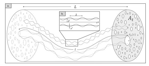
Figure 1: (a) The porous rock model is composed of a large number of sinusoidal and tortuous capillaries in the cylindrical representative elementary volume (REV). All the capillaries have the same tortuous length l (m) and their radii follow a fractal distribution. (b) The considered pore geometry corresponds to the one from Guarracino et al. (2014):  $\bar{r}$  is the average pore radius (m) while r' is the amplitude of the sinusoidal fluctuation (m), and  $\lambda$  is the wavelength (m).
