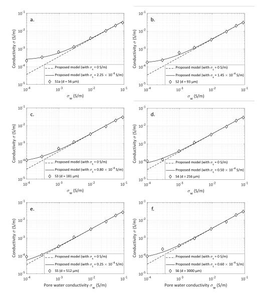
Figure 3: Electrical conductivity of different samples of glass beads (grains sizes are 56, 93, 181, 256, 512, and 3000  $\mu$ m for samples S1a, S2, S3, S4, S5, and S6, respectively) versus the fluid electrical conductivity for a constant porosity  $\phi = 40$  %. The datasets are from Bolève et al. (2007) and best fit parameters are given in Table 1.
