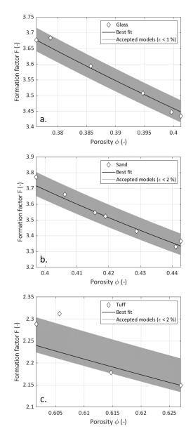
Figure 4: Formation factor of samples with different porosity values: (a) glass beads, (b) sand, and (c) tuff grains (Friedman and Robinson, 2002). The sets of adjusted model parameters a and  $\tau$  are given in Table 1.
