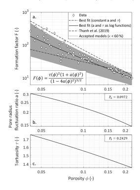
Figure 5: (a) Formation factors of a set of Fontainebleau sandstones versus porosity (the dataset is from Revil et al., 2014). Model parameters are given in Table 1. (b) and (c) a and  $\tau$  are defined as logarithmic functions of the porosity  $\phi$ .
