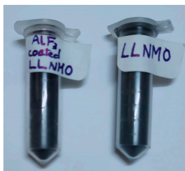
Figure 2. Photographs of pristine and \text{AlF}_3 -coated \text{Li}_{1.2}\text{Ni}_{0.2}\text{Mn}_{0.6}\text{O}_2 specimens.
