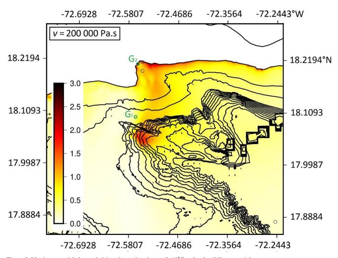
Figure 8: Maximum modeled wave height using a viscosity  $v = 2 \times 10^5$  Pa.s for the sliding material.
