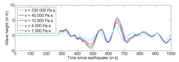
Figure 9: Time series calculated at synthetic gauge  $G_2$  located on the coast of the Bay of Jacmel (green circle in Fig. 8). This calculation uses a bathymetric grid with 25 m resolution.
