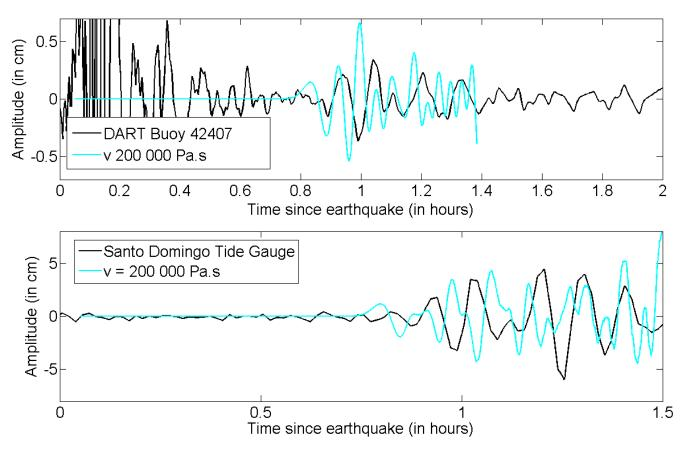
Figure 10: Comparison between observed and simulated water heights at the Santo Domingo tide gauge (top) and at DART buoy 42407 (bottom) for a dynamic viscosity  $\nu = 2 \times 10^5$  Pa.s.
