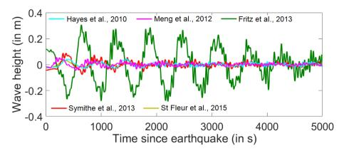
Figure 4: Water height comparison at a synthetic gauge located in the center of the Bay of Jacmel at a 30 m water depth. Calculation on a bathymetric grid uses a 30 second resolution.
