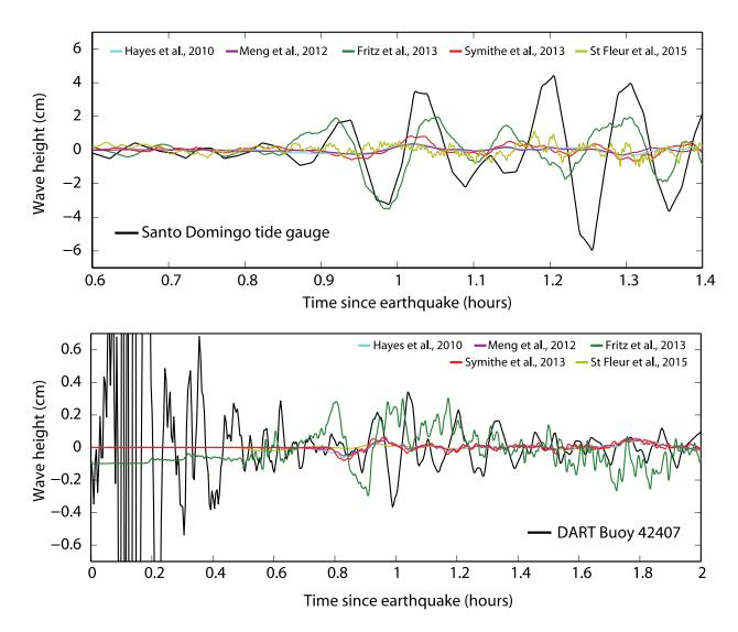
Figure 3: Comparison between observed and simulated water heights at the Santo Domingo tide gauge (top) and at DART buoy 42407 (bottom). Their locations are provided on Fig. 1. The high amplitude signal on the DART record before ~0.7 hours are seismic surface waves.
