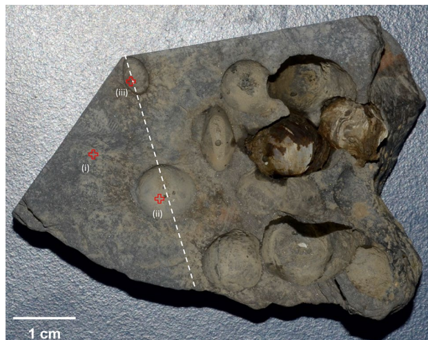
Figure 1. Photograph of a piece of siltstone collected from the middle reaches of the Kaladan River, western Myanmar, showing extensive pitting by Lignopholas fluminalis bivalves. The sample has been cut following the dashed line, and three locations were investigated by electron microscopy, namely (i) an area devoid of macroborings, the bottom of (ii) a large and (iii) a small macroboring, respectively.
