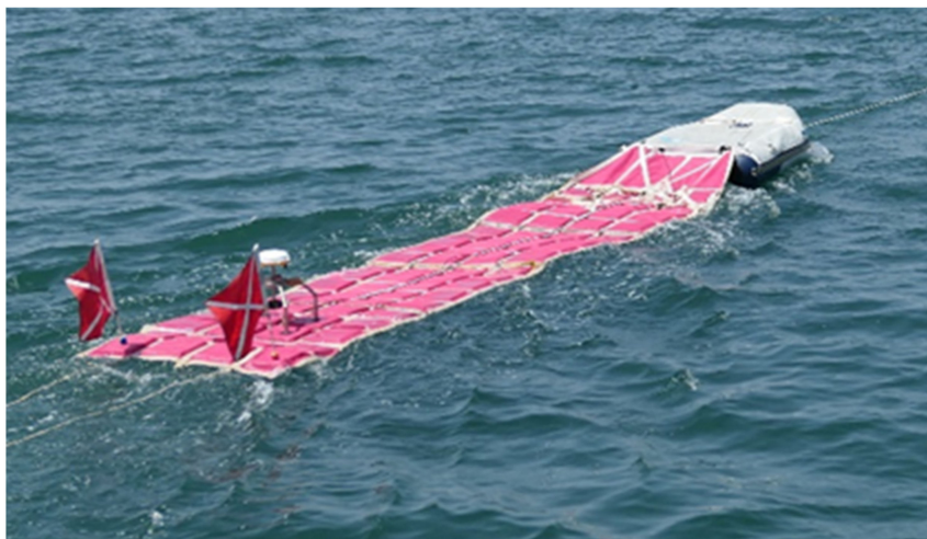
Figure 2. (a) A general drawing of the original CalNaGeo offshore towed carpet with a double inflatable boat in front (© M.Calzas—DT-INSU); (b) CalNaGeo coastal carpet in the Pertuis Charentais area.
