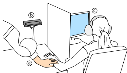
Fig. 2. Setup of the experiment. a) The robotic arm is hidden behind an opaque screen and touches the user’s forearm. b) A Kinect sensor tracks the user’s forearm to follow its arm anatomy. c) Participant wears both earphones emitting white noise and a noise-cancellation headphone to hide the sound of the robotic arm.
