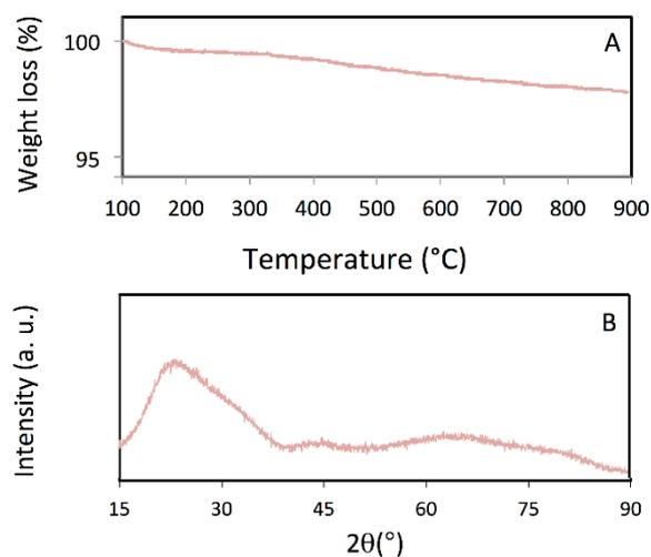
**Figure S12:** A: TGA profile and B: XRD pattern of the spent Ni<sup>0.5%</sup>@S. (The wide peak at  $15 < 2\theta < 30^\circ$  in B can be assigned to X-Ray diffraction by the amorphous silica walls).
