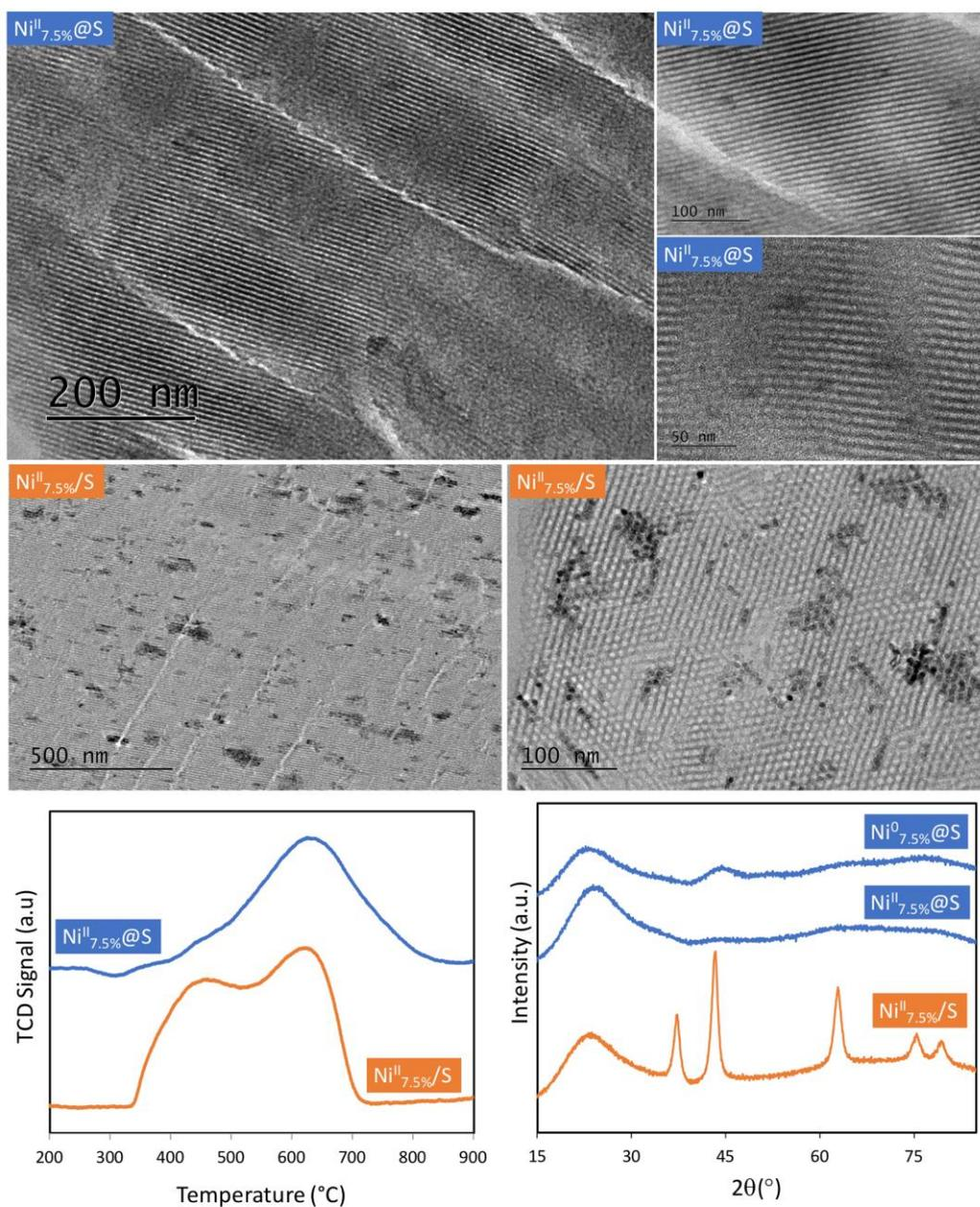
**Figure S18:** Summary of relevant results of  $\text{Ni}_{7.5\%}\text{@S}$  vs.  $\text{Ni}_{7.5\%}/\text{S}$  including TEM images, Ni reducibility ( $\text{H}_2$ -TPR) as well as XRD patterns revealing the effectiveness of the one-pot preparation method while increasing the metal loading.
