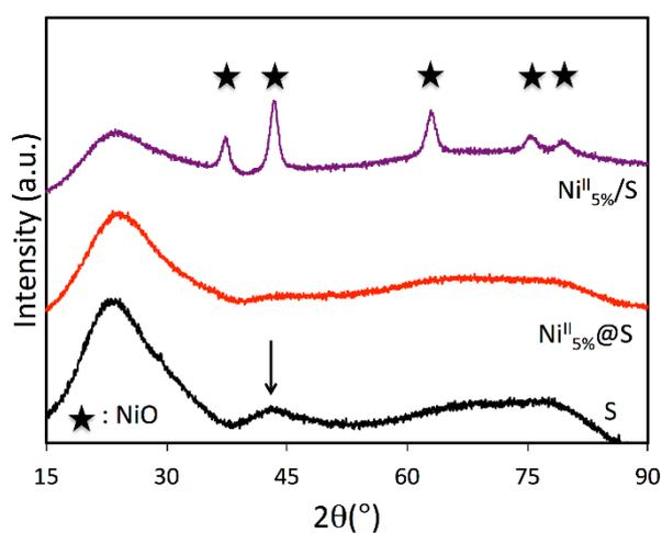
**Figure S3:** Wide angles XRD patterns of calcined  $\text{Ni}^{\text{II}}_{5\%}/S$ ,  $\text{Ni}^{\text{II}}_{5\%}@S$  and of the support,  $S$ . The wide peak between  $2\theta = 15\text{-}30^\circ$  is attributed to diffusion effects by the amorphous silica walls, whereas the wide peak at  $42^\circ$  in the  $S$  sample is attributed to the contribution of the PMMA sample holder.
