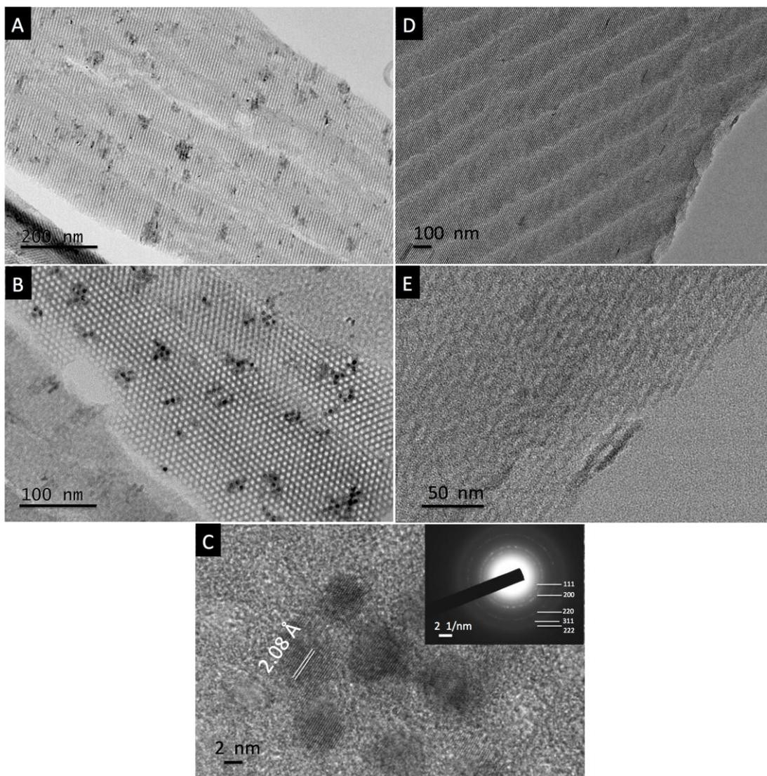
**Figure S6:** TEM images of microtomed  $\text{Ni}^{\text{II}}_{2.5\%}/\text{S}$  (A, B) and  $\text{Ni}^{\text{II}}_{2.5\%}\text{@S}$  (D and E) in their calcined state. HR-TEM image and SAED patterns of  $\text{Ni}^{\text{II}}_{2.5\%}/\text{S}$  (C).
