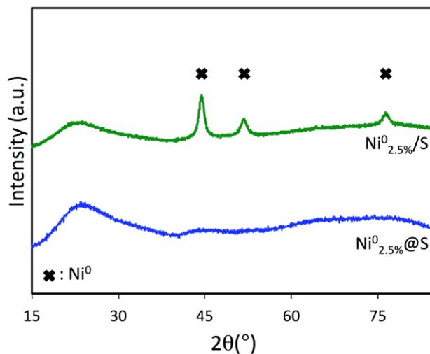
**Figure S9:** Wide angle XRD diffraction patterns of the  $\text{Ni}^{0.25\%}\text{-S}$  samples (reduced at  $650^\circ\text{C}$  for 2 h under a flow of  $30\text{ mL min}^{-1}$  of 5 vol.%  $\text{H}_2/\text{Ar}$ ). The wide peak between  $2\theta = 15\text{--}30^\circ$  is due to diffusion effects by the amorphous silica walls.
