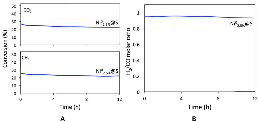
**Figure S16:** A) CH<sub>4</sub> and CO<sub>2</sub> conversions and B) H<sub>2</sub>/CO molar ratio reaction on Ni<sup>0</sup><sub>2.5%</sub>@S at 650°C for 12 h on stream under a GHSV of 960 L g<sup>-1</sup> h<sup>-1</sup>.
