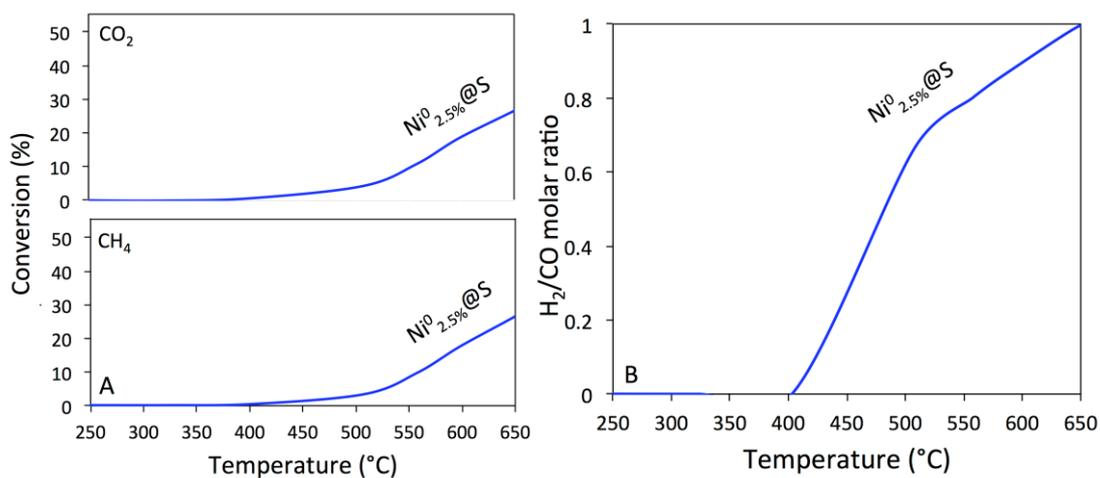
**Figure S15:** A) CH<sub>4</sub> and CO<sub>2</sub> conversions and B) H<sub>2</sub>/CO molar ratio in the DRM reaction on Ni<sup>0</sup><sub>2.5%</sub>@S as a function of temperature (GHSV of 960 L g<sup>-1</sup> h<sup>-1</sup>).
