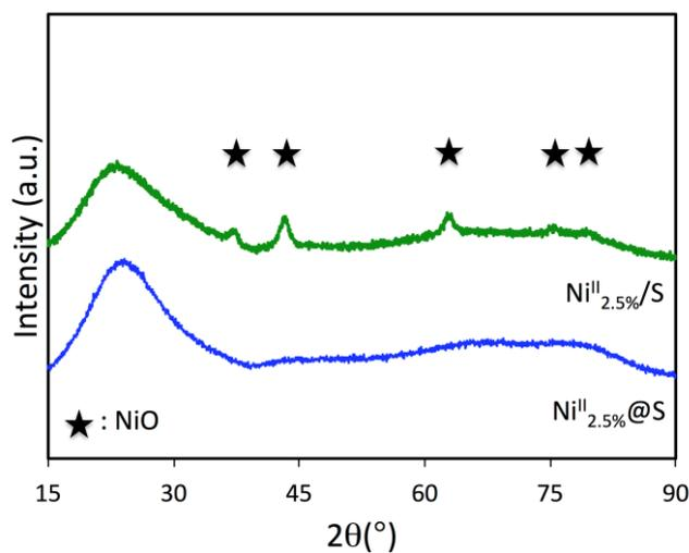
**Figure S4:** Wide angles XRD patterns of calcined  $\text{Ni}^{\text{II}}_{2.5\%}\text{-S}$  samples. The wide peak between  $2\theta = 15\text{-}30^\circ$  is attributed to diffusion effects by the amorphous silica walls.
