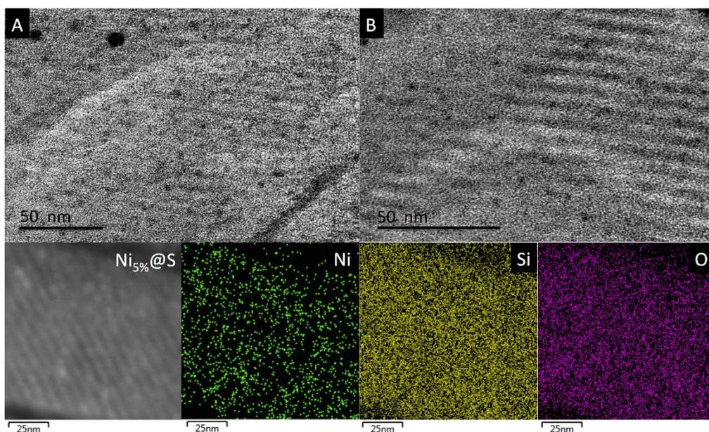
**Figure S13:** A and B: TEM images, STEM/HAADF and EDX/mapping (Ni in Green, Si in yellow and O in purple) acquired on typical areas of microtomed spent Ni<sup>0.5%</sup>@S ( $GHSV = 144 \text{ L g}^{-1} \text{ h}^{-1}$ ).
