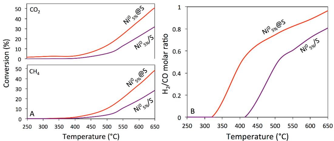
**Figure S14:** A: CH<sub>4</sub> and CO<sub>2</sub> conversions, and B: H<sub>2</sub>/CO molar ratio in the DRM reaction on Ni<sup>0</sup><sub>5%</sub>/S (purple) and Ni<sup>0</sup><sub>5%</sub>@S (red) at 650°C as a function of time on stream under a GHSV of 960 L g<sup>-1</sup> h<sup>-1</sup>.
