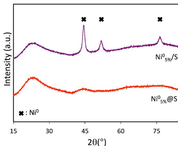
**Figure S8:** Wide angles XRD diffraction patterns of the  $\text{Ni}^0_{5\%}/\text{S}$  samples (reduced at  $650^\circ\text{C}$  for 2 h under a flow of  $30 \text{ mL min}^{-1}$  of 5 vol.%  $\text{H}_2/\text{Ar}$ ). The wide peak between  $2\theta = 15\text{-}30^\circ$  is assigned to the diffusion effects by the amorphous silica walls.
