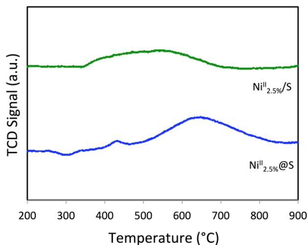
**Figure S5:**  $\text{H}_2$ -TPR profiles of the calcined  $\text{Ni}^{\text{II}}_{2.5\%}\text{-S}$  samples recorded with a  $\text{H}_2$  5 vol.%/Ar flow of  $30 \text{ mL min}^{-1}$  and a heating rate of  $10^\circ\text{C min}^{-1}$ .
