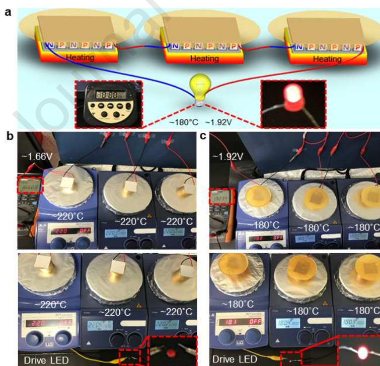
Figure 5. Tandem connection for practical cooling from high temperature and thermal energy utilization. (a) The scheme of BN50-PI50 for efficient high temperature heat dissipation and
