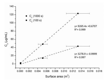
**Figure 5**: Concentration of dissolved silica at the solid-liquid interface after 100 seconds (squares) and 1000 seconds (circles) is reported versus surface area of the mesoporous silica films. Linear fit is showed. The point at the lowest surface value refers to dense silica while the porous samples have porosity values close to 62%. The surface area has been evaluated from EEP measurements with t-plot method, the error bars reported corresponds to an error on the surface value of 20%.
