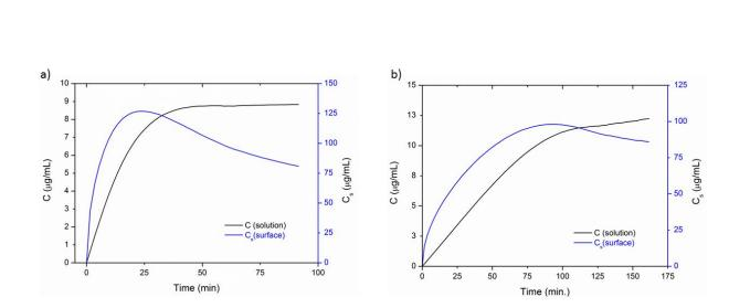
**Figure 4**: Bulk concentration (black line) and surface concentration (blue line) of dissolved silica for 1 cm<sup>2</sup> of mesoporous films having equivalent porous volume and template with **a**) CTAB, sample CT450-3 and **b**) Pluronic F-127, sample F450.
