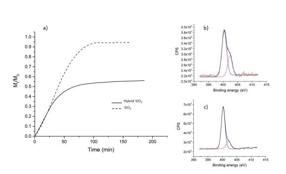
*Figure 10: a)* Dissolution curve of mesoporous hybrid organosilica (solid line, sample NCT130-1) and silica (dashed line, sample CT130-3) in PBS at 37°C. *b)* XPS peak of nitrogen from hybrid organosilica sample before dissolution, at 400 eV we observe the peak of free amine and at 402.5 eV the peak of amine interacting with silanols *c)* XPS peak of nitrogen from hybrid organosilica sample after 3h of dissolution, the peak at 402.5 decreased.
