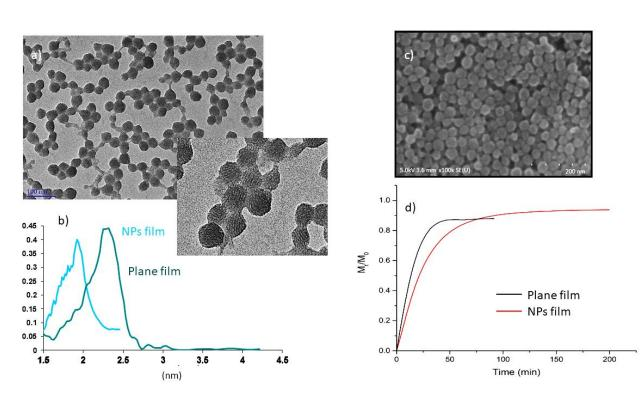
**Figure** 7: *a*) TEM image of mesoporous silica nanoparticles templated with CTAB, particles have size of 40 nm and a p6m structure (see blow-up) *b*) Pore size distribution of NPs film and mesoporous silica plane film CT130-1, obtained from EEP measurements *c*) SEM image of NPs film deposed on silicon *d*) Dissolution curves of NPs film and plane film in PBS at 37°C.
