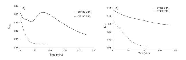
**Figure 13**: Refractive index at 632 nm of a mesoporous silica layer during dissolution in BSA solution at 37°C for **a**) sample washed to remove CTAB **b**) sample heated at 450°C to remove CTAB.
