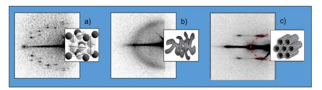
**Figure 2**: GI- SAXS patterns and the related mesostructures of mesoporous thin films obtained by dip-coating from solution at 26 °C and 30-35 % RH: **a**) Silica templated with CTAB, Pm3n structure **b**) Hybrid organosilica templated with CTAB, wormlike structure **c**) Silica, templated with Pluronic F-127, p6m structure. More detail with scale bar is provided in SI 1.
