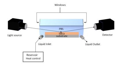
**Figure 1**: Experimental setup to investigate mesoporous silica thin film degradation in PBS by in situ ellipsometry. Both the liquid cell and the liquid reservoir are kept to a constant temperature of 37 °C.
