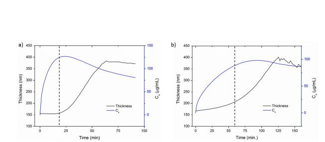
**Figure 6**: Thickness and  $C_s$  versus time for a) mesoporous silica CT450-3 film b) mesoporous silica F450 film.
