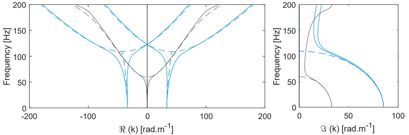
**Fig. S2. Theoretical dispersion relations.** The lossless (dashed line) and lossy (continuous line) wavenumbers (real part on left and imaginary parts on right) obtained for the two configurations with the fractional Maxwell-Voigt model presented in the main text. While the ZGV point disappears when adding losses the Dirac cone remains. The imaginary parts presented here have been used for the transparency of the lines of figure 2 and 3 in the main text.
