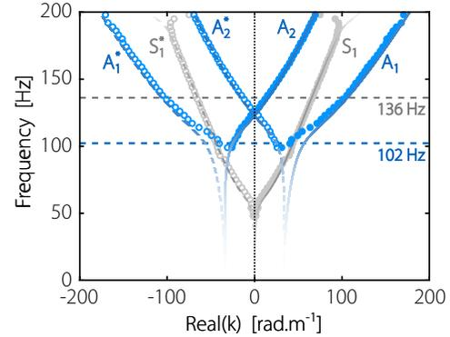
**Fig. 3. Fixed edges dispersion.** Experimental (symbols) and theoretical (solid lines) dispersion curves for a strip of width  $w = 50.6$  mm with fixed edges. Symmetrical modes (resp. anti-symmetrical) are labelled in gray (resp. blue). Similarly to Fig. 2.c, the transparency renders the ratio  $\text{Im}(k)/\text{Abs}(k)$  (see Supplementary Information). Filled gray and blue symbols correspond to extracted symmetrical and anti-symmetrical modes. Empty ones are obtained by symmetry.
