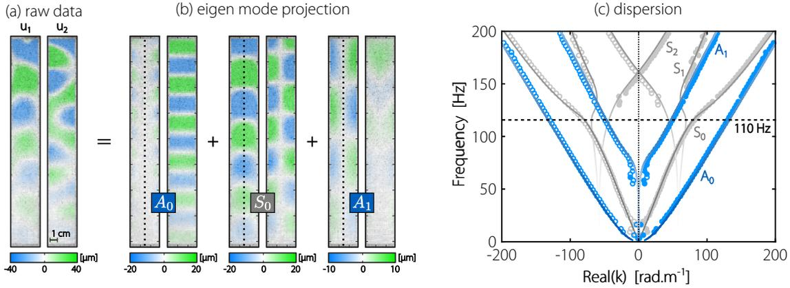
**Fig. 2. Free edges field maps and dispersion.** Here  $w = 39$  mm. (a) Real part of the raw displacements at 110 Hz and (b) the three corresponding singular vectors (see text). (c) Experimental (symbols) and analytical (solid lines) dispersion curves. Transparency renders the ratio  $\text{Im}(k)/\text{Abs}(k)$  (see Supplementary Information). Filled gray and blue symbols correspond to extracted symmetrical and anti-symmetrical modes. Empty ones are obtained by symmetry.
