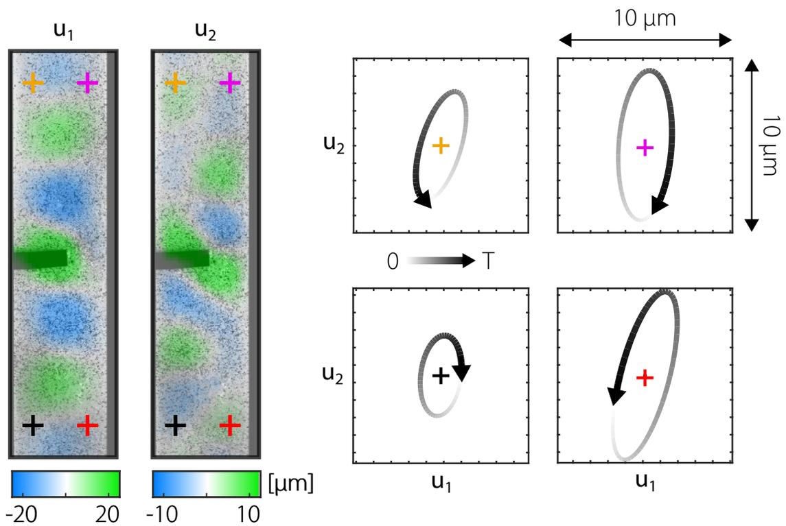
**Fig. S7. Fixed edges field patterns** (left) Snapshot of the field  $u_1$  (same data as figure 4 a) and  $u_2$  for a vertical excitation on the fixed edges strip. Represented over a full cycle the displacement measured on four different points exhibit elliptical displacements responsible for the selective excitations presented in figure 4. Note that those results have not been symmetrized as we do in the SVD in order to show the robustness of the process.
