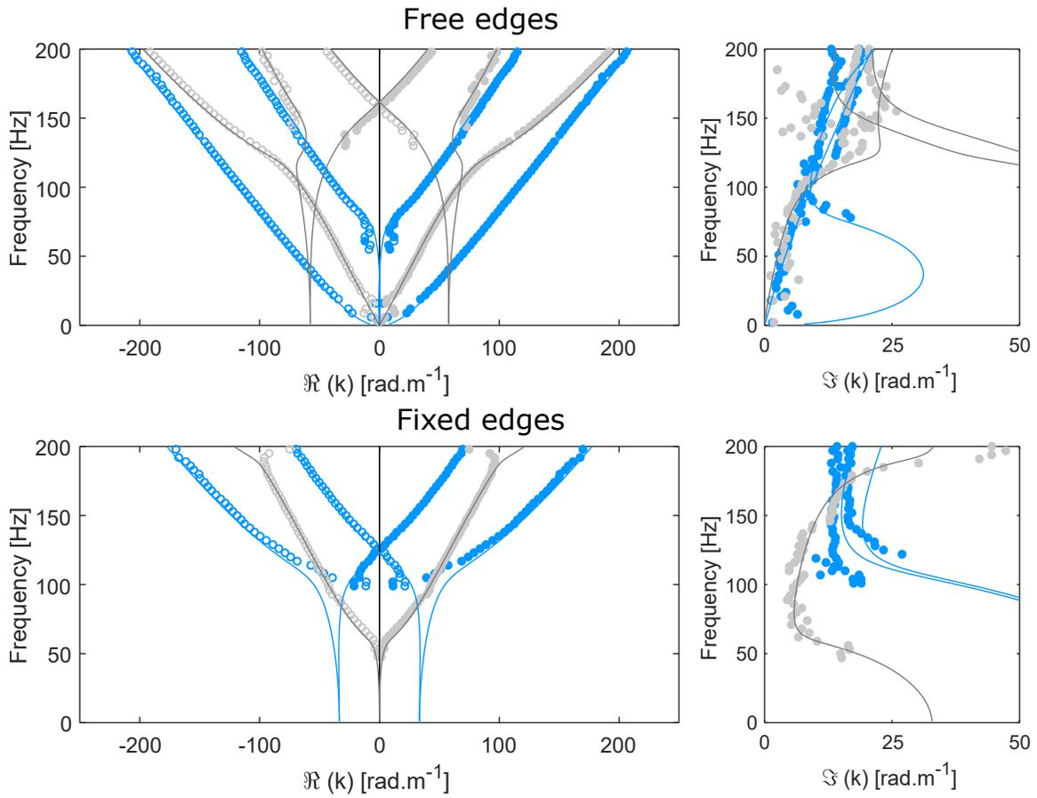
**Fig. S4. Experimental dispersion relations.** The real parts are the same as figure 2 and 3 of the main text, except that the theoretical line does not present transparency when the imaginary part increases. The extracted imaginary parts on the same experimental data are represented on the right.
