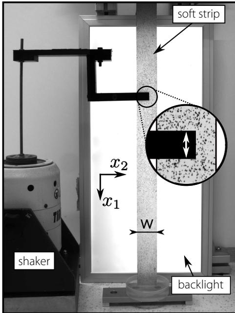
**Fig. 1. Experimental setup:** a soft elastic strip (of dimensions  $L = 600$  mm,  $w = 39$  mm,  $d = 3$  mm) seeded with dark pigments (for motion tracking purposes) is suspended. A shaker connected to a clamp induces in-plane displacement propagating along the strip.
