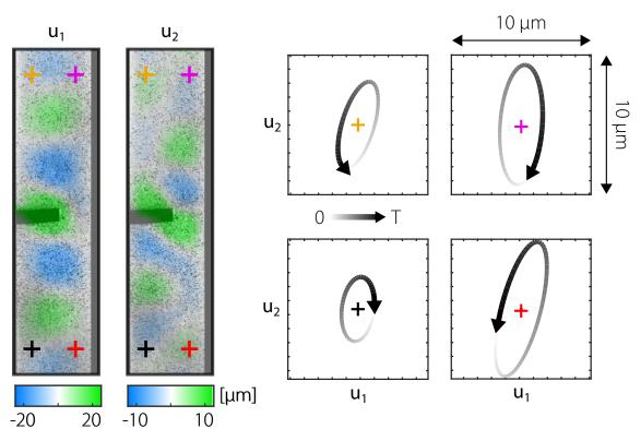
Fig. S7. Fixed edges field patterns (left) Snapshot of the field  $u_1$  (same data as figure 4 a) and  $u_2$  for a vertical excitation on the fixed edges strip. Represented over a full cycle the displacement measured on four different points exhibit elliptical displacements responsible for the selective excitations presented in figure 4. Note that those results have not been symmetrized as we do in the SVD in order to show the robustness of the process.
