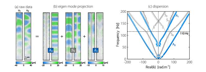
Fig. 2. Free edges field maps and dispersion. Here w=39 mm. (a) Real part of the raw displacements at 110 Hz and (b) the three corresponding singular vectors (see text). (c) Experimental (symbols) and analytical (solid lines) dispersion curves. Transparency renders the ratio Im(k)/Abs(k) (see Supplementary Information). Filled gray and blue symbols correspond to extracted symmetrical and anti-symmetrical modes. Empty ones are obtained by symmetry.
