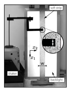
Fig. 1. Experimental setup: a soft elastic strip (of dimensions L=600 mm, w=39 mm, d=3 mm) seeded with dark pigments (for motion tracking purposes) is suspended. A shaker connected to a clamp induces in-plane displacement propagating along the strip.
