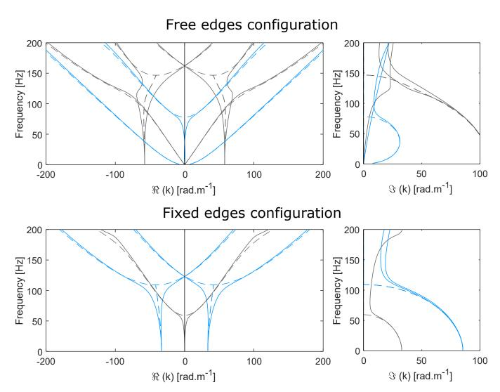
Fig. S2. Theoretical dispersion relations. The lossless (dashed line) and lossy (continuous line) wavenumbers (real part on left and imaginary parts on right) obtained for the two configurations with the fractional Maxwell-Voigt model presented in the main text. While the ZGV point disappears when adding losses the Dirac cone remains. The imaginary parts presented here have been used for the transparency of the lines of figure 2 and 3 in the main text.
