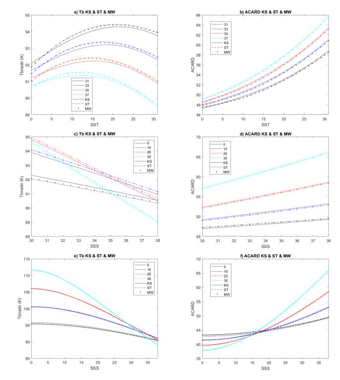
Figure 3: Tb at nadir (a, c, e) and pseudo dielectric constant Acard (b,d,f) plotted as (a,b) a function of SST, for various SSS values (in color), (c,d,e,f) a function of SSS for various SST values (in color) and (c,d) oceanic ranges of SSS and (e,f) the whole range of SSS, including fresh water. Tb and Acard are simulated with Klein and Swift (1977) (plain line), Meissner and Wentz (2012) (dotted line) and Somaraju and Trumpf (2006) (dashed line) dielectric constant models.
