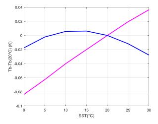
Figure 2: SST dependency of roughness induced Tb signal at a wind speed of 7 m.s<sup>-1</sup> and a SSS of 36, as simulated with the wind models used in Aquarius V3 (blue) and SMOS (magenta) retrievals. The y-axis reports the difference in modelled Tb at the temperature reported on the x-axis minus the modelled Tb at  $20 \, \text{C}$ .
