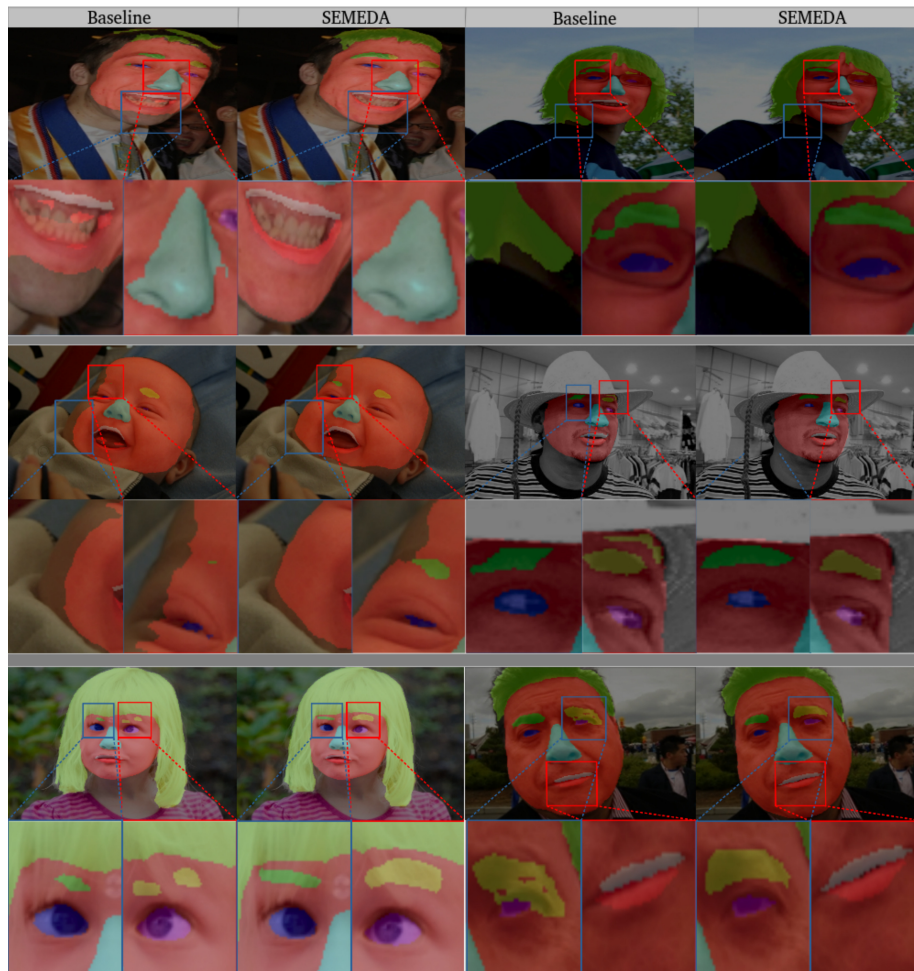
Figure 10: Examples of predicted segmentation masks on HELEN dataset, and comparison between a baseline Deeplab v3+ model trained with PPCE and SEMEDA. SEMEDA produces better shaped predictions compared with the baseline.
