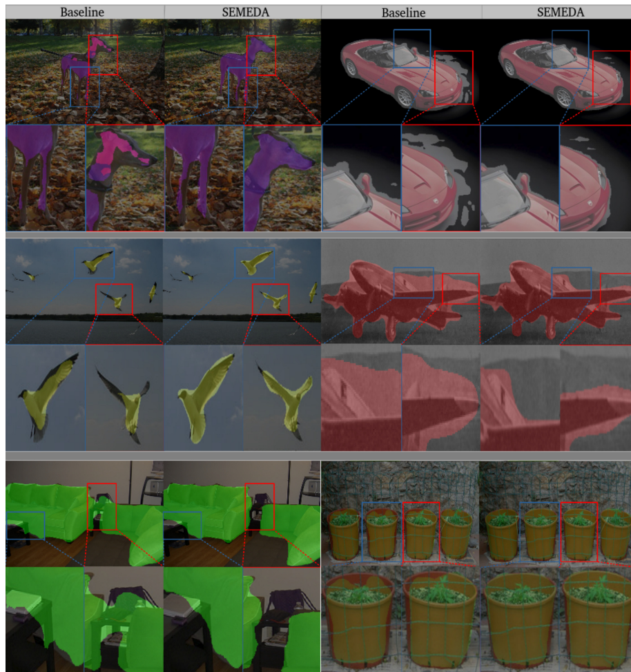
Figure 8: Examples of predicted segmentation masks on VOC 2012 dataset, and comparison between a baseline Deeplab v3+ model trained with PPCE and SEMEDA. SEMEDA produces better shaped predictions compared with the baseline.
