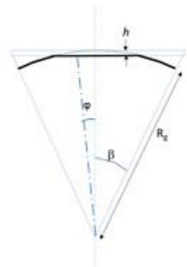
Fig. A.1: The granules under compression progressively transforms into polyhedra. At the end of the process, the voids are mostly on the vertices and on the edges of the polyhedra.
