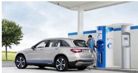
Figure 25. Mercedes GLC F-Cell SUV light vehicle: mild-hybrid type with a 50 kW FCS.
