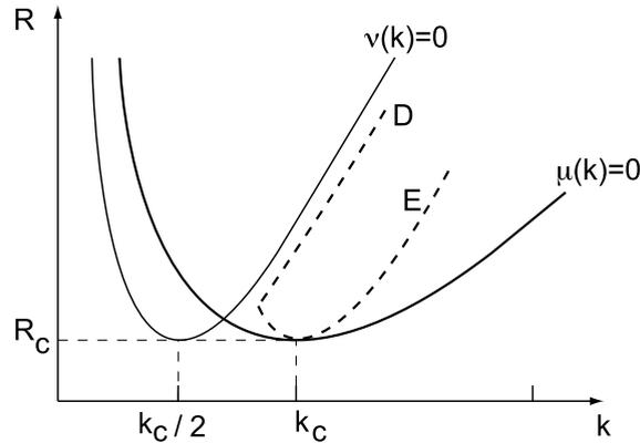
**Figure 2.** Neutral stability curves  $\mu(k) = 0$  for the mode of wave number  $k$  and  $\nu(k) = 0$  for the mode of wave number  $2k$ . The domain of stable stationary patterns is limited by the Eckhaus instability (E) and the drift bifurcation (D).
