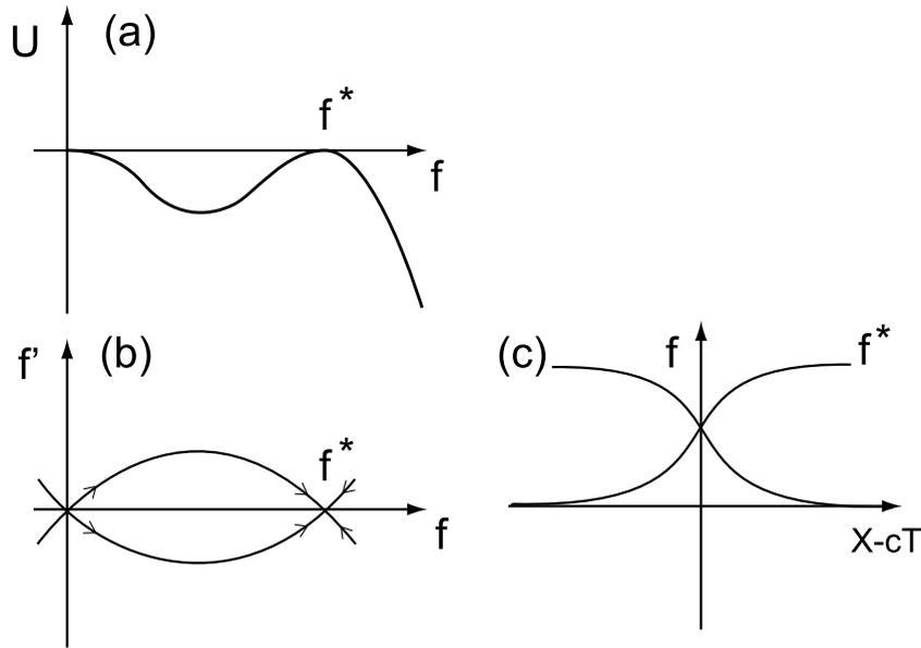
**Figure 3.** Kink-type solutions of (24). (a) The shape of the potential  $U(f)$  given by (25) for  $\lambda = \lambda^*$ . (b) Phase space of (24) with the two heteroclinic orbits that connect  $(0,0)$  and  $(f^*,0)$ . (c) The corresponding kink-type solutions (28).
