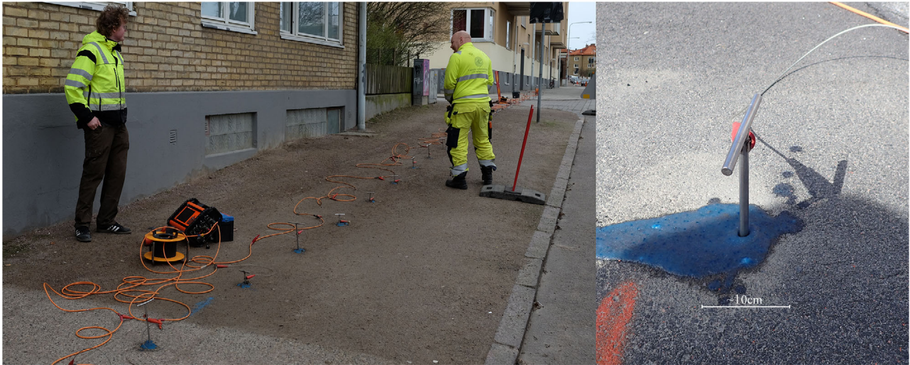
Figure 1 Sketch showing part of the ERT layout, and photo of a drilled hole with an electrode and blue starch gel (Johnson Revert Optimum®) used to reduce contact resistance.
