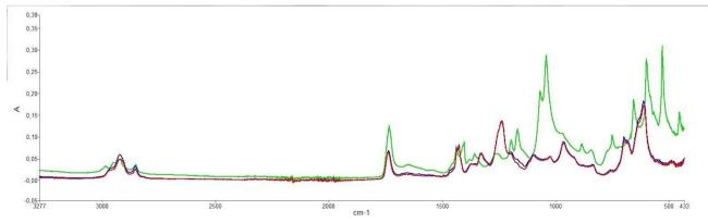
**Figure 3** Typical Fourier transformed infrared spectroscopy of a polyvinyl-chloride polymer packaging with (green spectrum) and without (blue and red spectrum) polyvinylidine-chloride.
