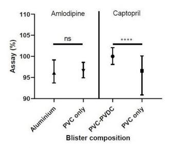
**Figure 4** Medians of drug assays with IQRs as a function of the drug and the blister composition; \*\*\*\*p<0.0001. PVC, polyvinyl-chloride; PVDC, polyvinylidine-chloride; ns, non-statistically significant.
