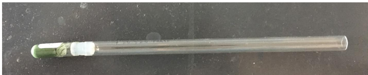
Figure 15 : picture of the sample NMR tube with its extension for introduction in the relaxometers.
