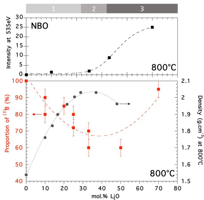
**Fig. 7:** Evolution of the intensity of the peak at 535 eV related with NBOs (black colored squares), the proportion of  $^{13}\text{B}$  (red colored squares) and the density<sup>50</sup> at 800°C (grey colored circles) as a function of  $\text{Li}_2\text{O}$  content. The dashed lines are a guide for the eyes.
