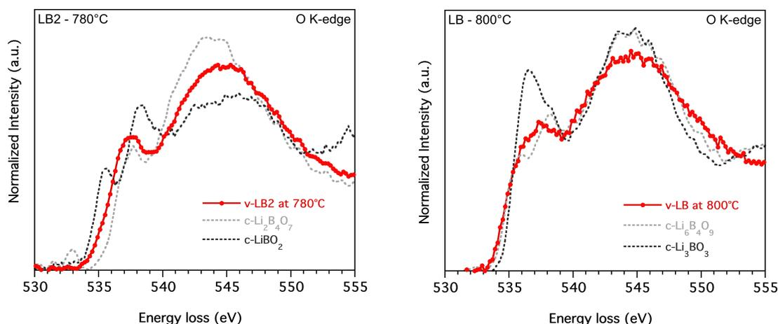
**Fig. 5:** Left: O K-edge XRS spectra of LB2 melt (red points) accompanied with two crystalline phases:  $\text{Li}_2\text{B}_4\text{O}_7$  (grey) and  $\text{LiBO}_2$  (black). Right: O K-edge XRS spectra of LB melt (red points) accompanied with two crystalline phases:  $\text{Li}_6\text{B}_4\text{O}_9$  (grey) and  $\text{Li}_3\text{BO}_3$  (black).
