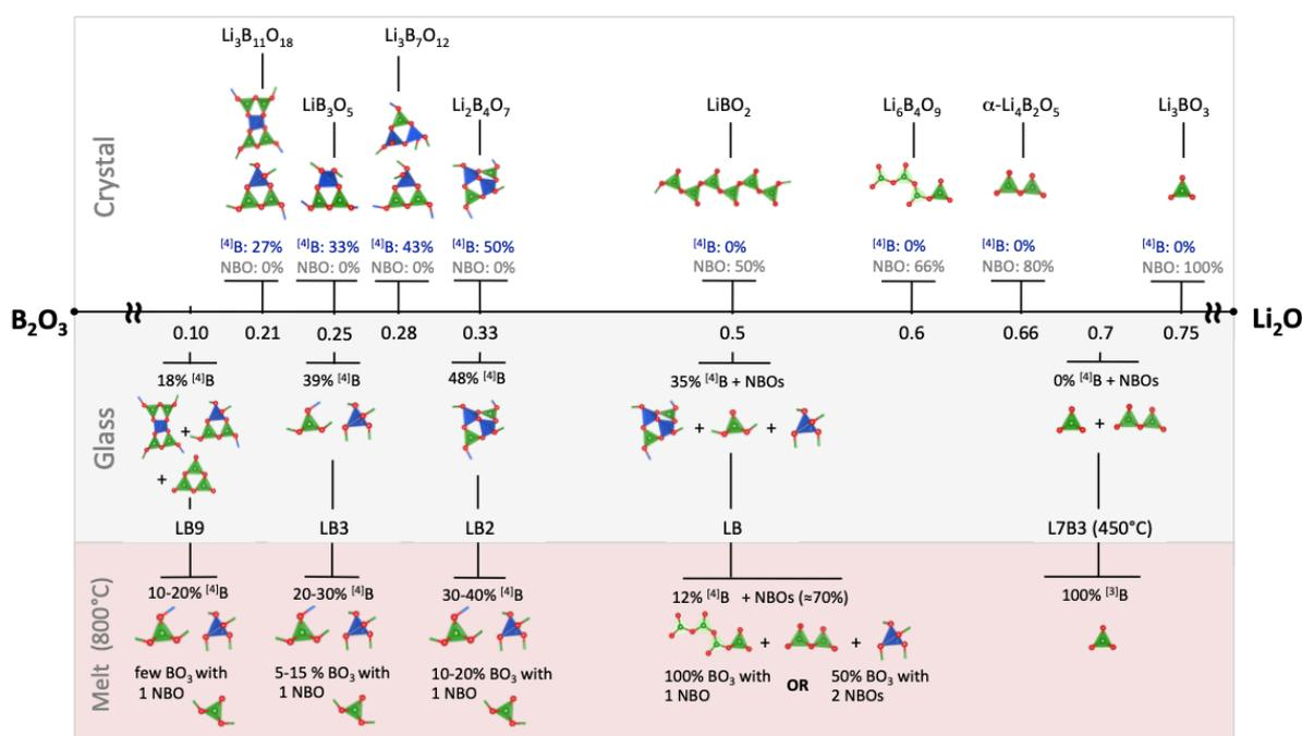
**Fig. 6:** Summary of the superstructural units found in crystalline phases (top), in glasses at room temperature (grey-shaded area) and in the melt (red-shaded area) for the  $\text{Li}_2\text{O}-\text{B}_2\text{O}_3$  system.
