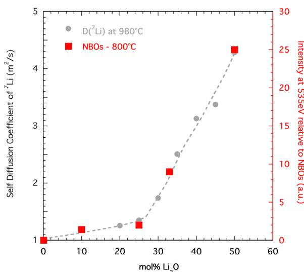
**Fig. 8:** Comparison between the intensity of the peak at 535eV at 800°C, which is indicative of the proportion of NBOs (red squares) and the self-diffusion coefficient of  $^7\text{Li}$  measured by NMR<sup>52</sup> at 975°C (grey circles) as a function of  $\text{Li}_2\text{O}$  content.
