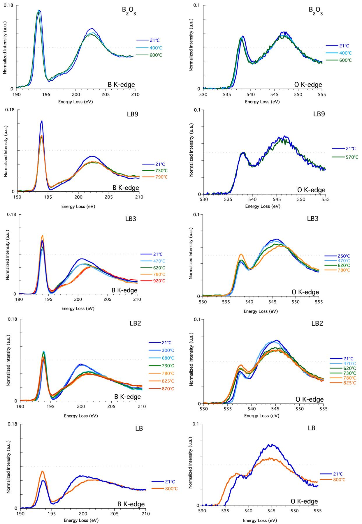
**Fig. 2:** *in situ* B K-edge (left) and O K-edge (right) XRS spectra of  $v$ - $B_2O_3$ , LB9, LB3, LB2 and LB glasses as a function of temperature. All the spectra were measured in the levitation chamber with the exception of the B K-edge of LB9 at room temperature, which has been measured in a standard sample holder.
