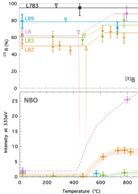
**Fig. 3:** Evolution of the proportion of  $^{[3]}\text{B}$  (top) and the intensity at 535eV (bottom) as a function of temperature and  $\text{Li}_2\text{O}$  content: LB9 (cyan), LB3 (green), LB2 (orange), LB (pink) and L7B3 from reference<sup>7</sup> (black). The plain and dashed colored lines are a guide for the eyes, and the arrows are indicative of the glass transition temperatures of the different glasses.<sup>13</sup>
